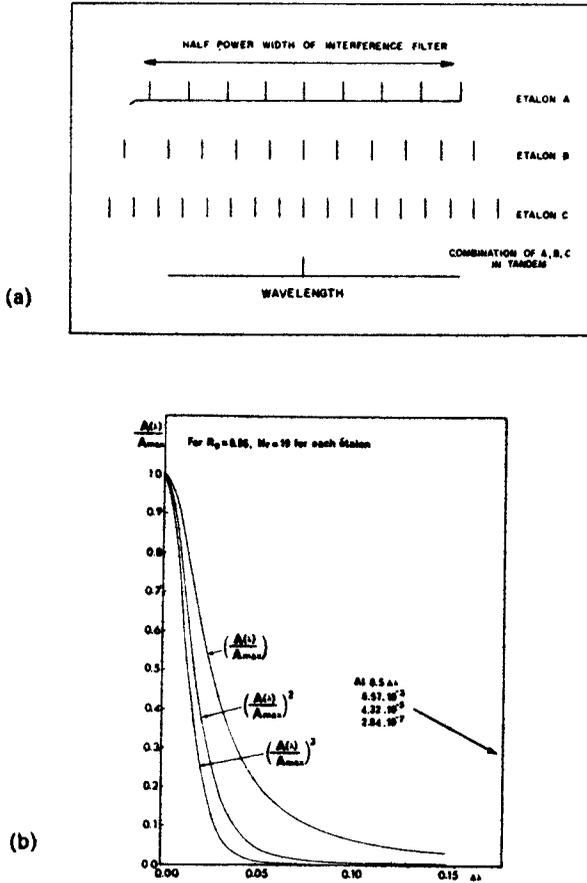
**Figure 6(a).** Principle of PEPSIOS. Interference filter F plus three etalons A, B and C in vernier spacer ratio in series. **(b)** Transmission profile of a single etalon compared with two and three identical etalons in series (Meaburn 1976).
