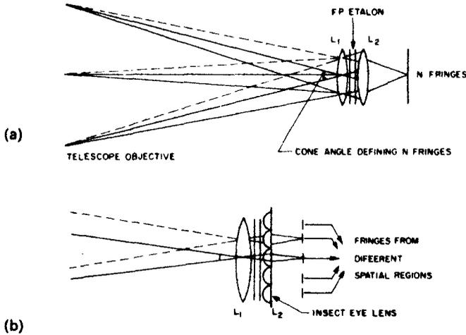
**Figure 4(a).** Telecentric use of Fabry-Perot.  $N$  gives number of fringes in the cone angle.
