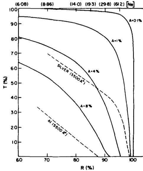
Figure 2. Transmission vs reflectivity of FP etalon for reflecting layers of different absorption values.
