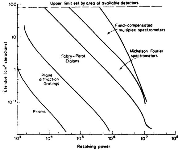
**Figure 1.** Etendue (i.e. luminosity) vs resolving power for different spectrometer systems. (from James and Sternberg 1966).
