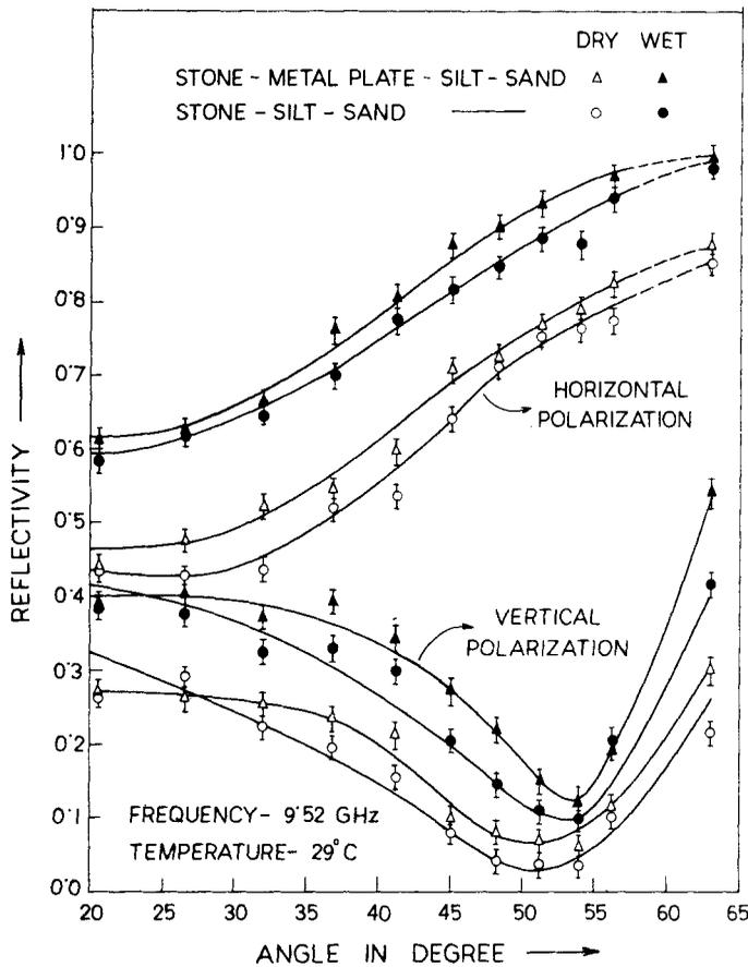
**Figure 5.** Angular variation of reflectivity for two sets of subsurface condition (comparison).
