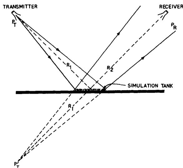
Figure 2. Schematic representation showing reflection from the mocked-up model surface.
