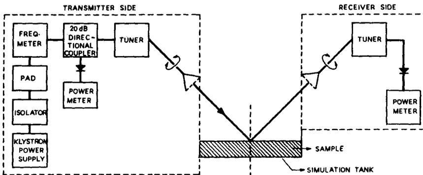
Figure 1. Block diagram of bistatic scatterometer system.
