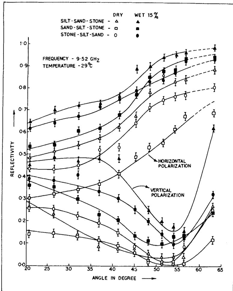
Figure 3. Angular variation of reflectivity for various stratification of subsurface materials.
