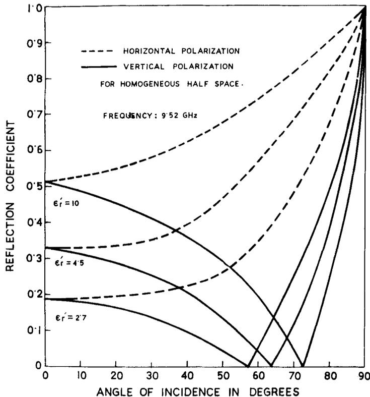
**Figure 6.** Angular variation of reflection coefficient for a plane wave incident on a semi-infinite media with  $\epsilon_r = 2.7, 4.5, 10$  and  $\mu_r = 1$ .
