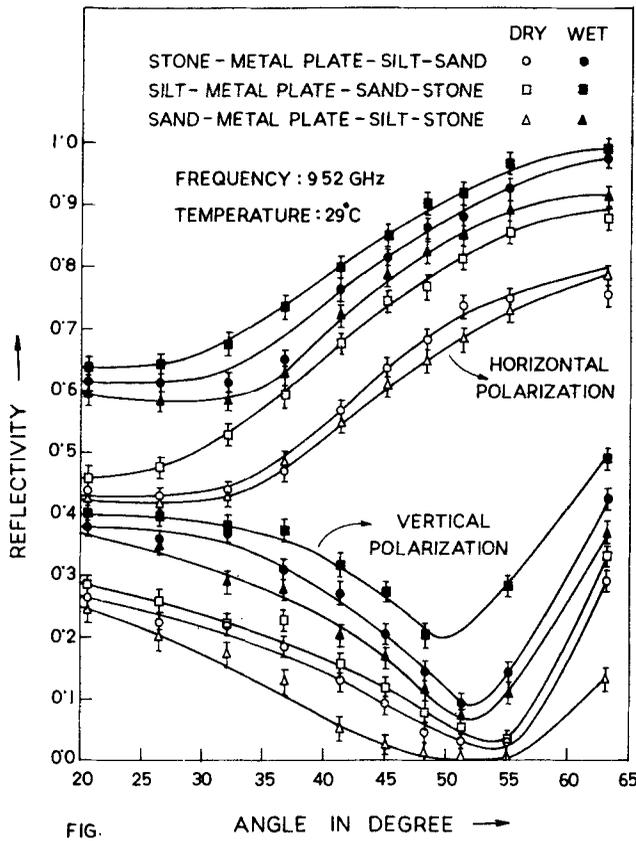
Figure 4. Angular variation of reflectivity for various stratifications of subsurface materials with buried metal plate.
