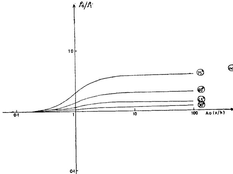
Figure 5. The relation between  $\rho_0/\rho_1$  and angle of inclination of the sides of an anticline obtained using a simple three-electrode (AMN) system.
