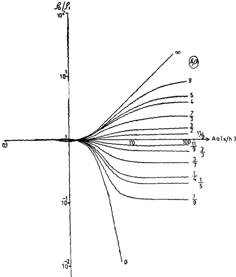
Figure 4. Apparent resistivity master curves for sounding over a two-layered earth obtained with a second horizontal derivative ( $\partial^2 U/\partial x^2$ ) measuring set-up.
