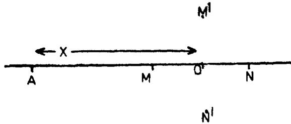
Figure 1. Placement of source and measuring electrodes for obtaining the second vertical derivative ( $\partial^2 U / \partial Z^2$ ).
