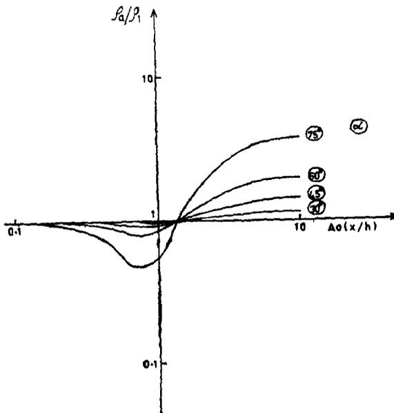
Figure 3. Apparent resistivity curves  $\rho_a$  obtained by sounding  $(\partial^2 U/\partial Z^2)$  over an anticlinal structure of infinite resistivity showing the variation in  $\rho_2/\rho_1$  with the inclination of the sides ( $\alpha$ ).
