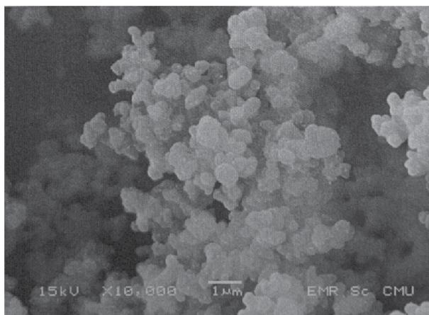
**Figure 2.** SEM image of MIP-TPPO synthesized by using Sty and EGDMA.
