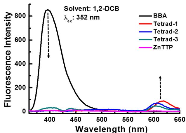
**Figure 3.** Emission spectra ( $\lambda_{\text{ex}} = 352$  nm) and (OD  $\lambda_{\text{abs}} = 0.1$ ) of equiabsorbing compositions of **BBA**, **ZnTTP** and **Tetrad-1**, **Tetrad-2**, and **Tetrad-3** in 1,2-DCB.
