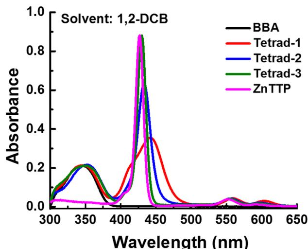
**Figure 2.** Absorption spectra of the specified compounds in 1,2-DCB.
