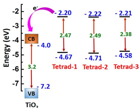
**Figure 5.** Schematic energy level diagram.
