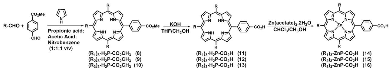
**Scheme 1.** Synthetic scheme of carboxylic acid substituted BBA-zinc porphyrins.
