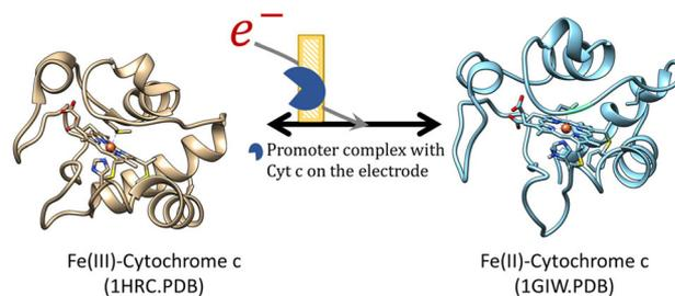
**Figure 4.** Schematic representation of electrochemical reduction of Fe(III)-cytochrome *c* (Crystal structure 1HRC.PDB) forming Fe(II)-cytochrome *c* (Crystal structure 1GIW.PDB) immobilized on the gold electrode containing monolayer of the Schiff base complex as promoter for electrochemistry.
