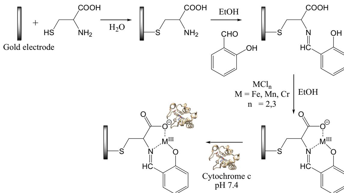
**Figure 1.** Schematic representation of electrode modification with M-Schiff base complex and cytochrome c, where M = Fe(III), Mn(III), Cr(III).
