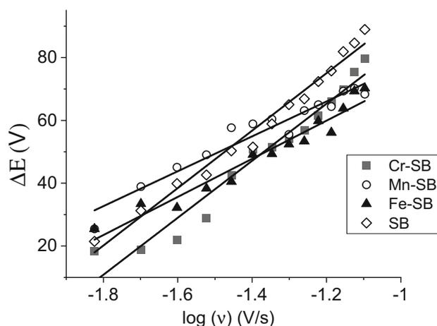
**Figure 7.** Plot of  $\Delta E_p$  vs.  $\log v$  for Cytochrome c on modified Au electrode containing monolayer of Schiff base (SB) and its metal complexes (M-SB) in 40 mM phosphate buffer, pH 7.4, 40 mM KCl at room temperature in nitrogen saturated solution at different scan rates [M=Fe(III), Mn(III), Cr(III)].
