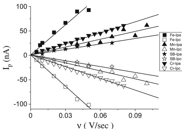
**Figure 6.** Plot of peak current vs. scan rate of Schiff base conjugated Cyt c on gold electrode in 40 mM phosphate buffer, pH 7.4, 40 mM KCl at room temperature in nitrogen saturated solution at different scan rates. The electrode area is  $0.0314 \text{ cm}^2$ .
