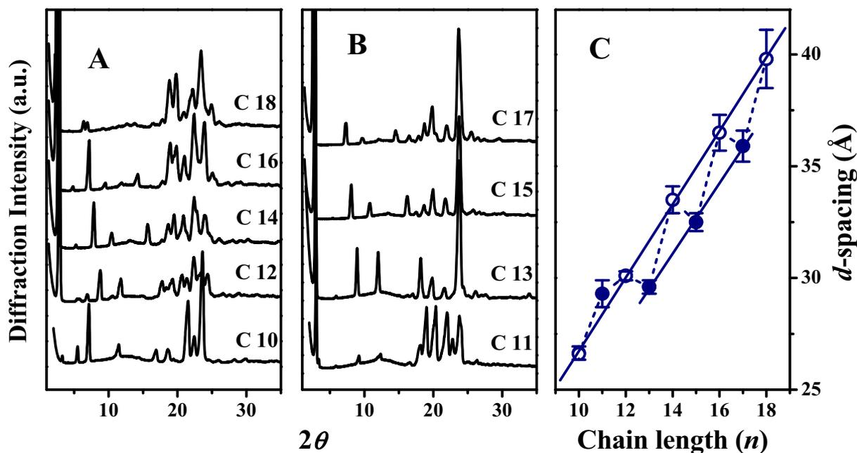
**Figure 7.** Powder X-ray diffraction patterns of DAAOHs with different saturated acyl chains (A, B) and dependence of  $d$ -spacings on the chain length (C). The number of C-atoms in the acyl chain is indicated against each PXRD profile. Filled symbols, odd chainlength compounds; open symbols, even chainlength compounds. The solid lines in C represent linear least-squares fit of the data. Data corresponding to C11 compound was omitted from the linear fit as it is an outlier.
