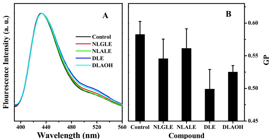
**Figure 8.** (A) Emission spectra of Laurdan in stratum corneum model (SCM) lipid mixture and SCM containing 20 mol% NLGLE, NLALE, DLE, or DLAOH. (B) Comparison of Laurdan GP values for the different samples. See text for details.
