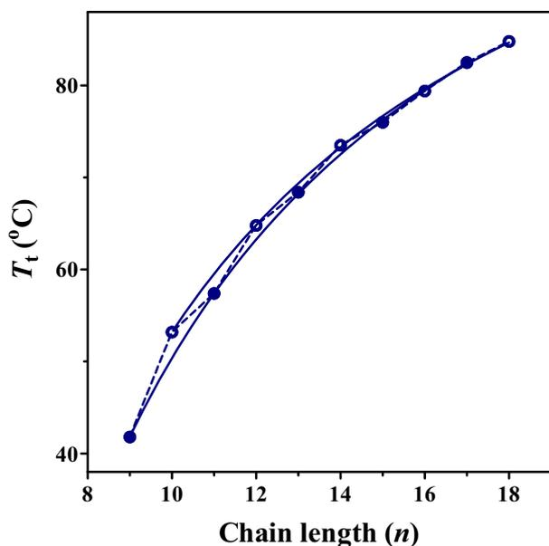
**Figure 4.** Chainlength dependence of solid-liquid phase transition temperatures ( $T_t$ ) of DAAOHs. Solid lines correspond to a nonlinear least-squares fit of the transition temperatures to Eq. 8. Filled symbols, odd chainlength compounds; open symbols, even chainlength compounds.
