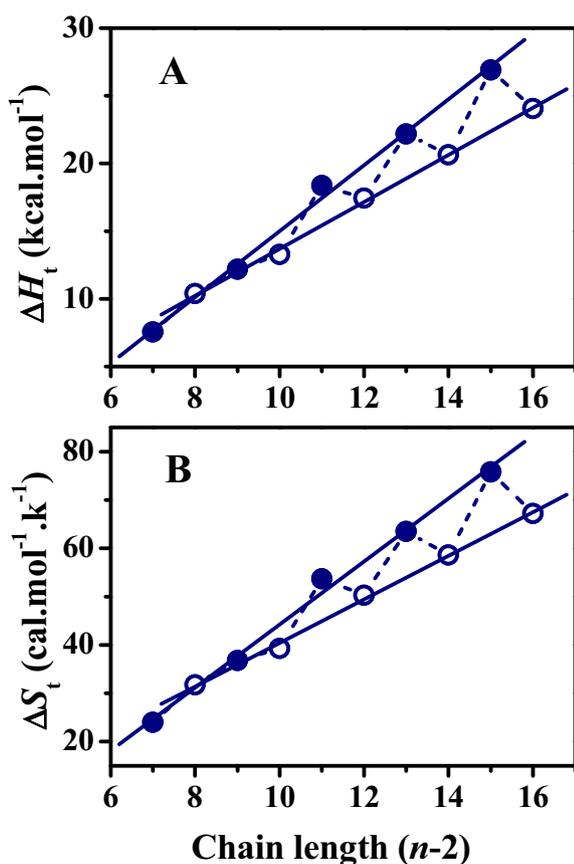
**Figure 3.** Chainlength dependence of transition enthalpy (A) and transition entropy (B) of dry DAAOHs from the first heating scans. Values of  $\Delta H_t$  and  $\Delta S_t$  were plotted against the number of methylene units ( $n-2$ ). Filled symbols, odd chainlength compounds; open symbols, even chainlength compounds. Solid lines correspond to linear least-squares fits of the data.
