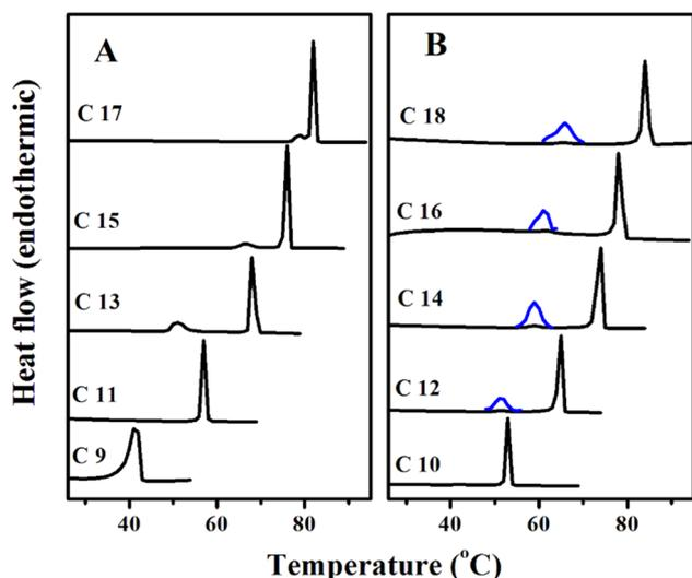
**Figure 2.** DSC first heating thermograms of dry DAAOHs with odd (A) and even (B) number of C-atoms in the acyl chain. The number of C-atoms is indicated against each thermogram. Less-intense minor transitions of even-chain DAAOHs are vertically expanded 15 times and shown in blue color.
