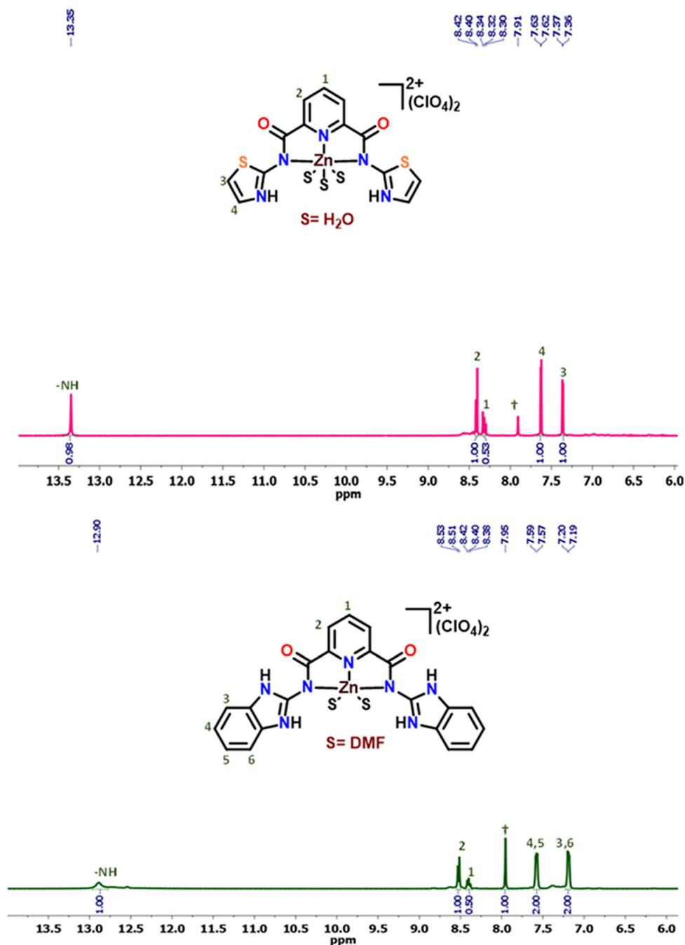
**Figure 2.**  $^1\text{H}$  NMR spectra of complexes **1** (pink trace) and **2** (green trace) recorded in  $\text{DMSO-d}_6$  where † represents  $-\text{C}(\text{O})\text{H}$  proton of the DMF molecule(s).
