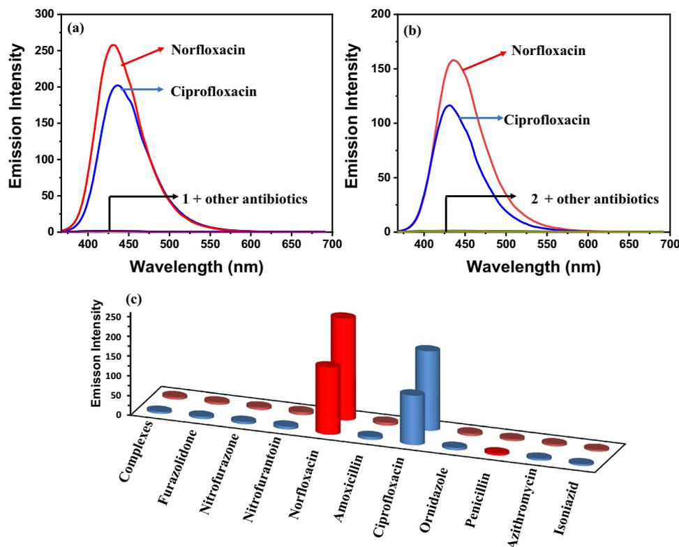
**Figure 4.** Change in the emission spectra of complexes (20  $\mu\text{M}$ ) (a) **1** and (b) **2** in the presence of 5 equiv. of different antibiotics. (c) Bar diagram showing emission spectral enhancement for zinc complexes in the presence of different antibiotics: **1** (430 nm, red bars) and **2** (430 nm, blue bars). All studies were performed in EtOH containing 2%  $\text{CH}_3\text{CN}$  ( $\lambda_{\text{ex}} = 350 \text{ nm}$ ).
