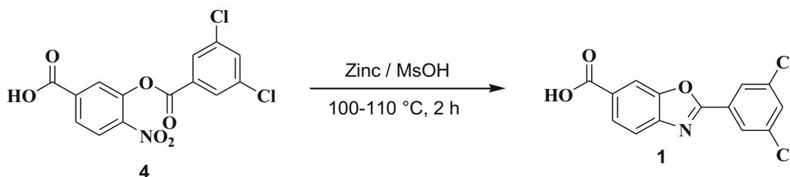
**Scheme 2.** Synthesis of Tafamidis (**1**) from 3-(3,5-dichlorobenzoyloxy)-4-nitrobenzoic acid (**4**).
