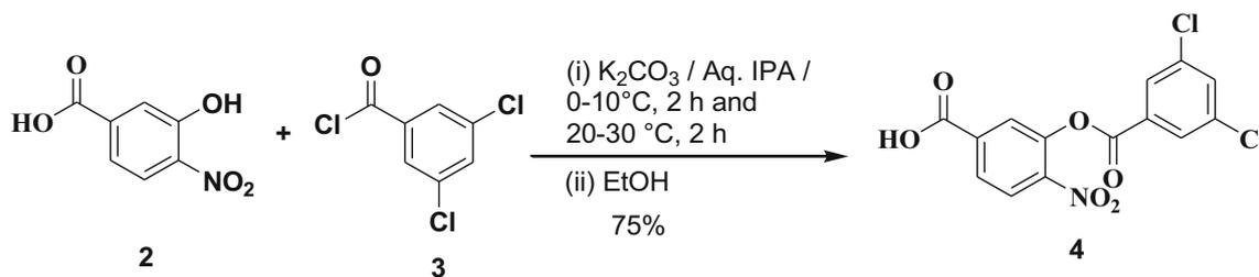
**Scheme 1.** Synthesis of 3-(3,5-dichlorobenzoyloxy)-4-nitrobenzoic acid (**4**) from 3-hydroxy-4-nitrobenzoic acid (**2**).
