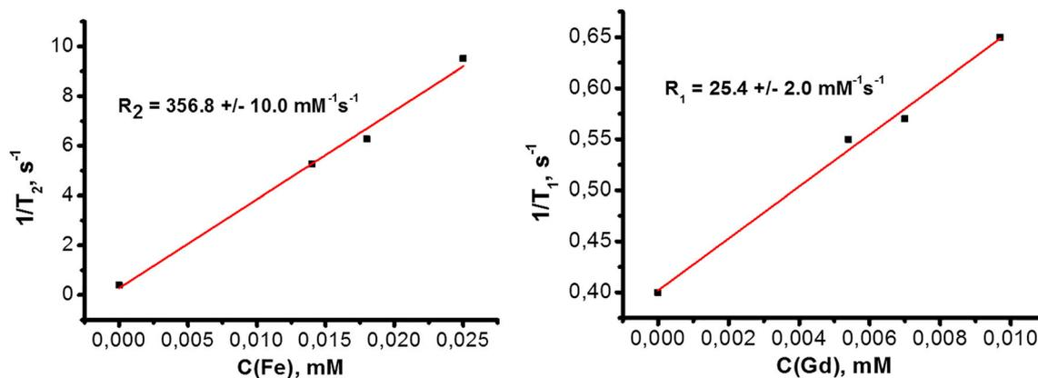
**Figure 2.** Reciprocal T<sub>2</sub> and T<sub>1</sub> vs. Fe and Gd concentrations (1.5 T medical NMR whole-body scanner). PVA mass fraction 4.5%.
