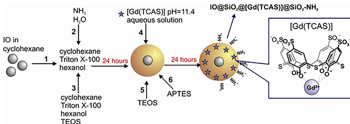
**Scheme 1.** Schematic representation of synthesis of IO@SiO<sub>2</sub>@[Gd(TCAS)]@SiO<sub>2</sub>-NH<sub>2</sub> nanoparticles.
