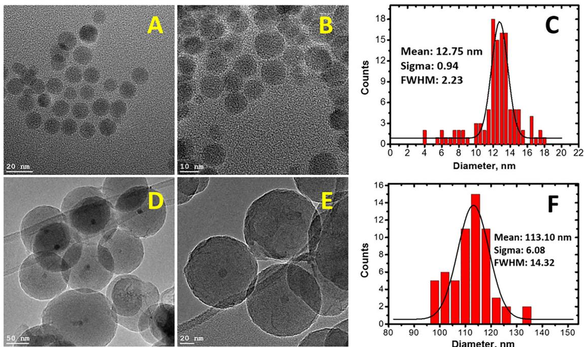
**Figure 1.** TEM images of oleate-coated iron-oxide nanoparticles (panels A and B), size distribution diagram of iron-oxide nanoparticles (panel C). TEM images of IO@SiO<sub>2</sub>@[Gd(TCAS)]@SiO<sub>2</sub>-NH<sub>2</sub> nanoparticles (panels D and E), size distribution of IO@SiO<sub>2</sub>@[Gd(TCAS)]@SiO<sub>2</sub>-NH<sub>2</sub> nanoparticles (panel F).
