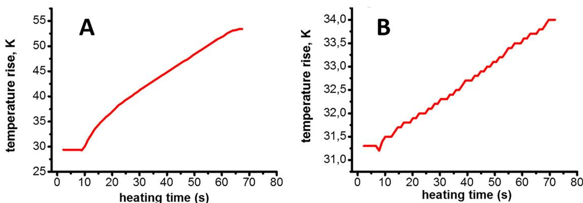
**Figure 3.** Panel A: heating curve of oleate-coated iron-oxide nanoparticles in DMSO. Panel B: heating curve of IO@SiO<sub>2</sub>@[Gd(TCAS)]@SiO<sub>2</sub>-NH<sub>2</sub> aqueous dispersion.
