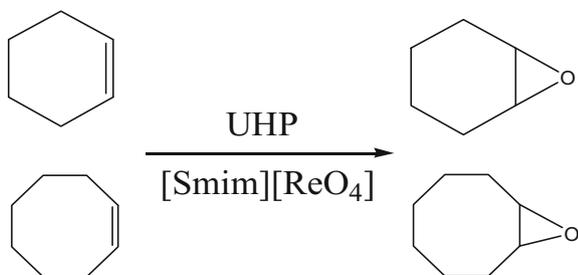
**Figure 3.** Olefin epoxidation in IL [Smim][ReO<sub>4</sub>].
