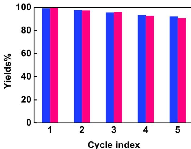
**Figure 5.** The recycling efficiency of IL  $[\text{Smim}][\text{ReO}_4]$  affects the yields with the substrates of cyclohexene (blue) and cyclooctene (pink).
