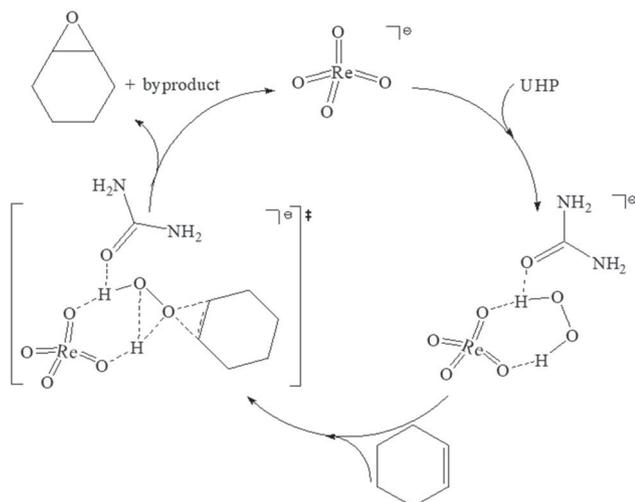
**Scheme 2.** Mechanism of the epoxidation of olefins catalysed by  $[\text{Smim}][\text{ReO}_4]$ .
