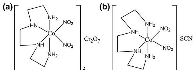
**Scheme 2.** (a) Structure of  $[\text{Co}(\text{trien})(\text{NO}_2)_2]_2\text{Cr}_2\text{O}_7$ . (b) Structure of  $[\text{Co}(\text{trien})(\text{NO}_2)_2]\text{SCN}$ .
