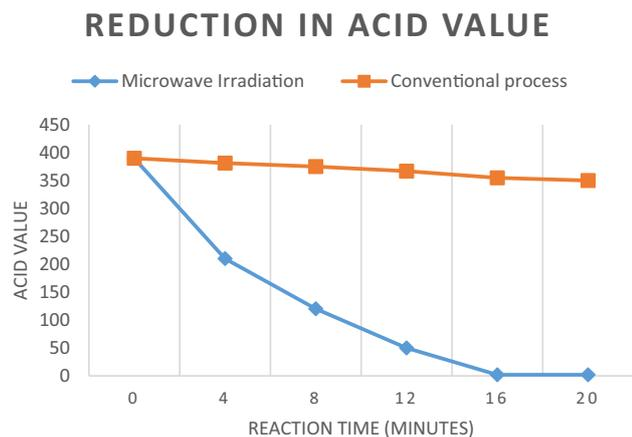
**Figure 6.** Reduction in acid value in microwave and conventional process.
