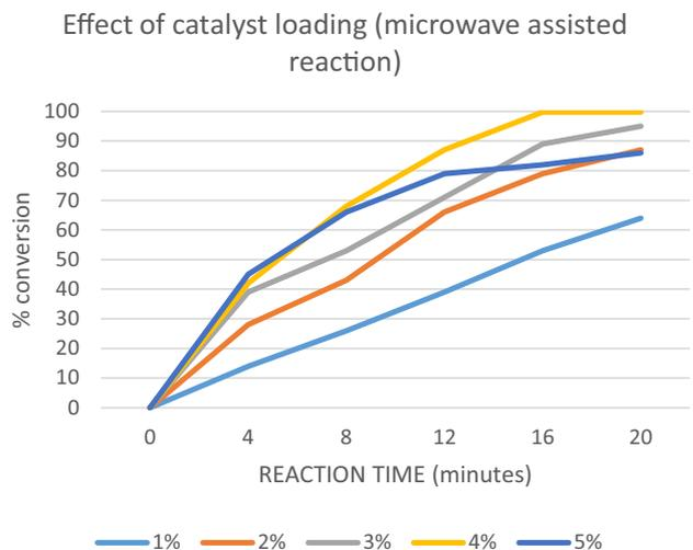
**Figure 3.** Effect of catalyst loading on % conversion in microwave-assisted reaction.
