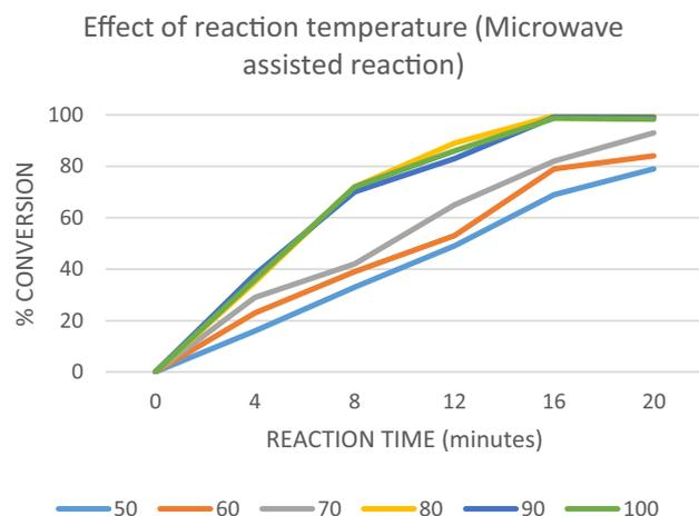
**Figure 4.** Effect of reaction temperature on % conversion in microwave-assisted process.
