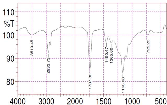
**Figure 8.** IR spectra of tricapyrylin.
