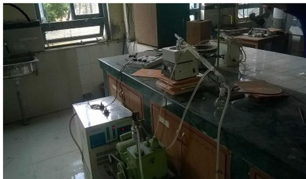
**Figure 1.** Experimental arrangement for conventional synthesis of tricaprylin.
