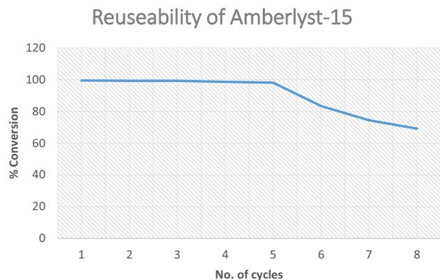
**Figure 7.** Reusability of Amberlyst-15 for 8 cycles of esterification reaction between caprylic acid and glycerol.
