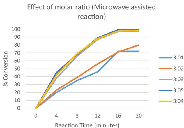
**Figure 2.** Effect of molar ratio of caprylic acid:glycerol on % conversion in microwave assisted reaction.
