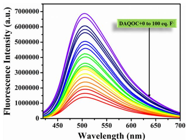
Figure 3. Emission spectral change of DAQOC ( $4 \times 10^{-5}$  M) upon the addition of 0-100 equivalents of  $F^-$  in acetonitrile.
