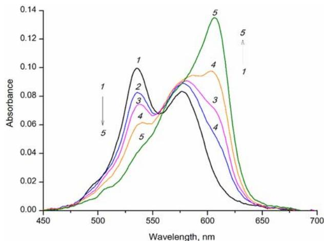
**Figure 4.** Absorption spectra of OXEC in an aqueous solution at different concentrations of HSA:  $c_{\text{HSA}} = 0$  (1); 0.99 (2), 1.98 (3), 5.8 (4), 24 (5)  $\mu\text{M}$ .
