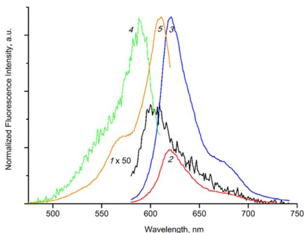
**Figure 5.** Fluorescence (curves 1–3), normalized fluorescence excitation spectra (curves 4, 5) of OXEC ( $\lambda_{\text{ex}} = 570$  nm,  $\lambda_{\text{reg}} \sim 620, 630$  nm) at different concentrations of HSA:  $c_{\text{HSA}} = 0$  (1, 4), 0.99 (2), 24 (3, 5)  $\mu\text{M}$ .
