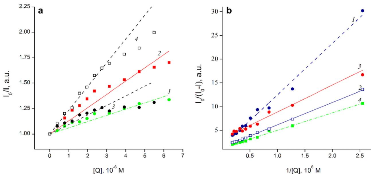
**Figure 7.** Stern-Volmer (a) and Lehrer-Leavis (b) plots according to the quenching of synchronous fluorescence of HSA (1, 2) and BSA (3, 4) with OXEC, at  $\Delta\lambda = 15$  nm (1, 3) and at  $\Delta\lambda = 60$  nm (2, 4).
