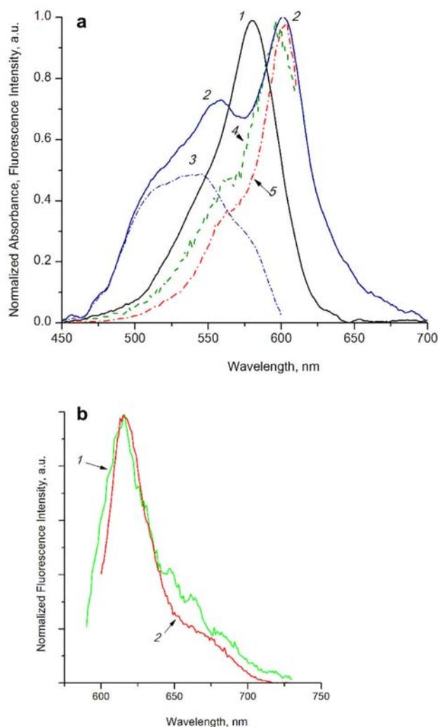
**Figure 2.** (a) Normalized absorption (1, 2, 3) and fluorescence excitation spectra (4, 5) of OXEC in polar ethanol (1, 4) and in nonpolar 1,4-dioxane (2, 3, 5); (b) normalized fluorescence spectra of OXEC in ethanol (1) and in nonpolar 1,4-dioxane (2).
