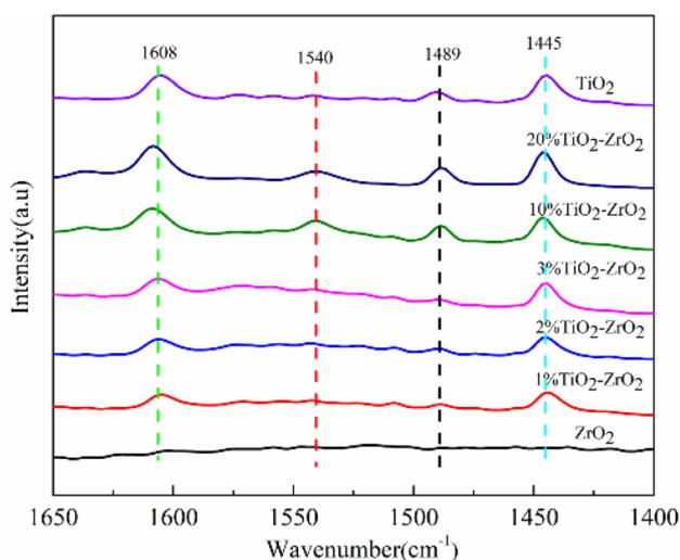
**Figure 3.** Py-IR spectra of the catalysts.
