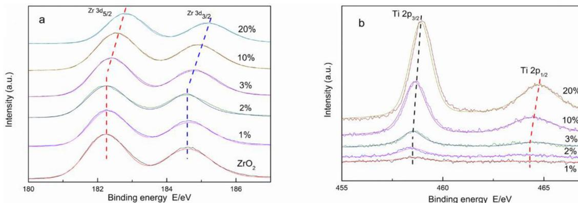
**Figure 2.** Zr 3d (a) and Ti 2p binding energy spectra (b) of the catalysts.
