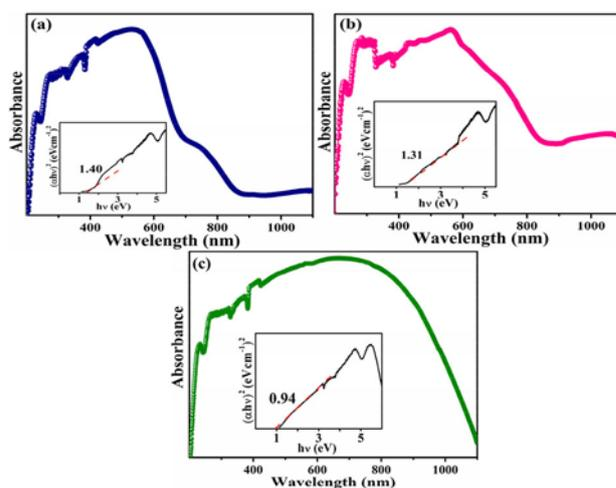
**Figure 5.** Shows UV-visible spectra of (a)  $\text{CuSbS}_2$ , (b)  $\text{Cu}_3\text{SbS}_3$  and (c)  $\text{Cu}_3\text{Sb}_{0.50}\text{Bi}_{0.50}\text{S}_3$ , respectively. Insets show the corresponding Tauc plots for bandgap calculation.
