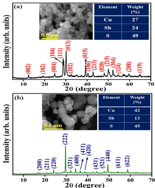
**Figure 1.** Shows PXRD patterns of the products from the refluxing reaction of  $[\text{Cu}(\text{tu})_3]\text{Cl}$  and  $[\text{Sb}(\text{tu})_2]\text{Cl}_3$  complexes in 1:1 molar ratio in (a) ethanolamine and (b) ethylene glycol for 90 min. Insets show SEM image, energy dispersive spectral analysis.
