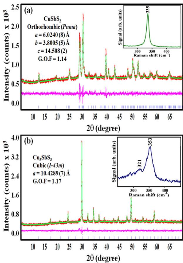
**Figure 2.** Shows Le Bail refinement of PXRD patterns of (a)  $\text{CuSbS}_2$  and (b)  $\text{Cu}_3\text{SbS}_3$  (Redline-experimental data; green line-calculated profile; pink line-difference profile. Vertical bars indicate Bragg positions). Inset shows their room temperature Raman spectra.
