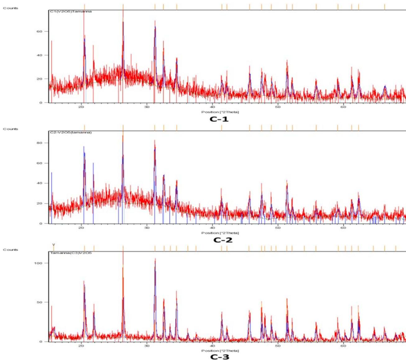
**Figure 2.** X-ray diffraction patterns of  $V_2O_5$  nanoparticles (C-1, C-2 and C-3).
