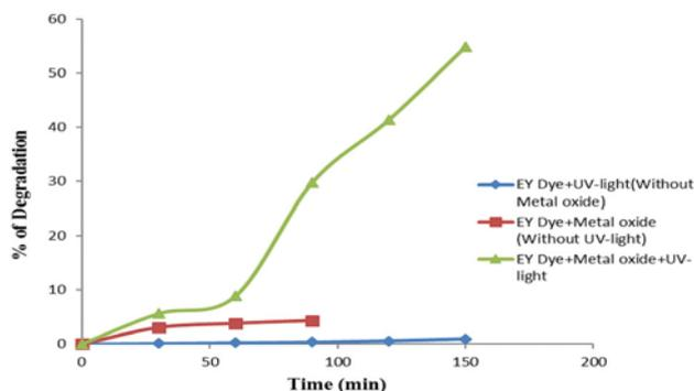
**Figure 7.** Photocatalytic degradation (%) of EY dye with time.
