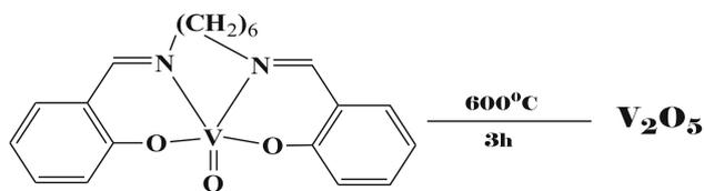
**Figure 1.**  $V_2O_5$  nanoparticles prepared from VO(Sal-Hn-Sal) complex.
