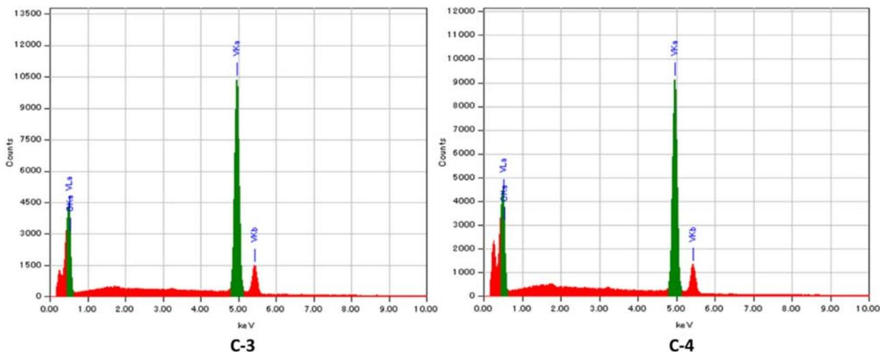
**Figure 4.** EDS image of synthesized V<sub>2</sub>O<sub>5</sub> nanoparticles, C-3 and C-4.
