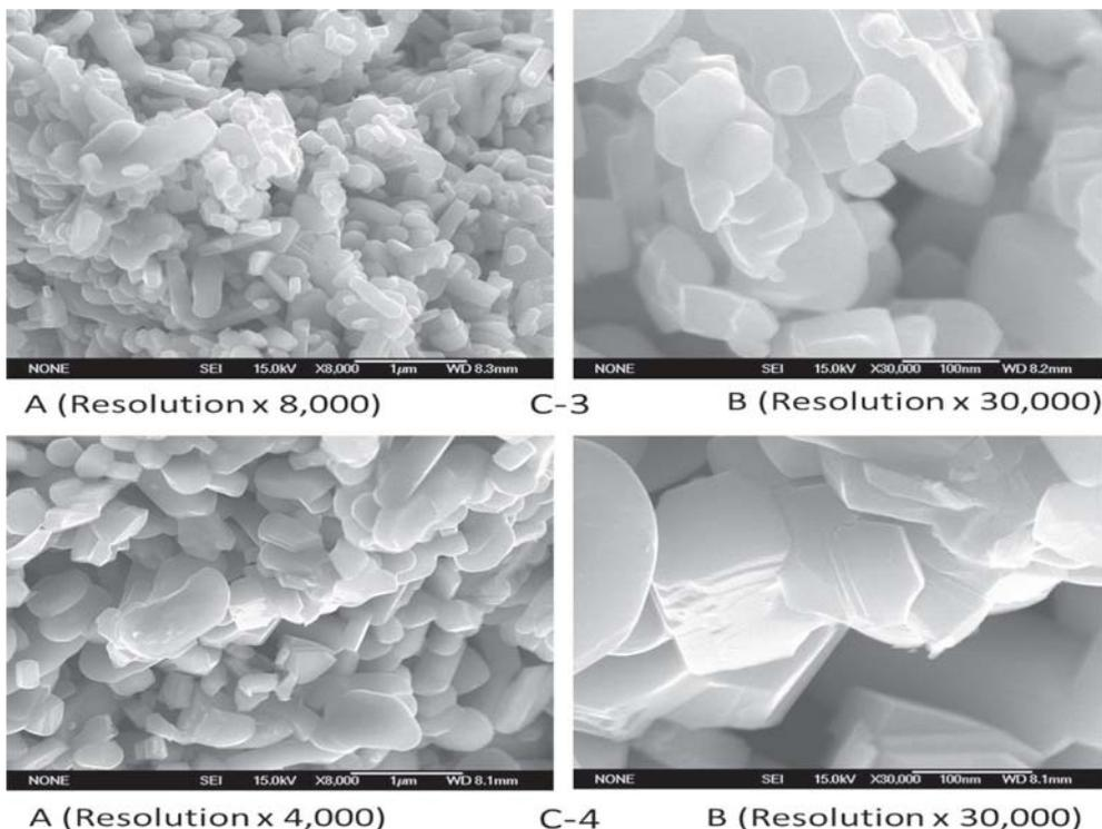
**Figure 3.** SEM images of V<sub>2</sub>O<sub>5</sub> nanoparticles, C-3 and C-4.
