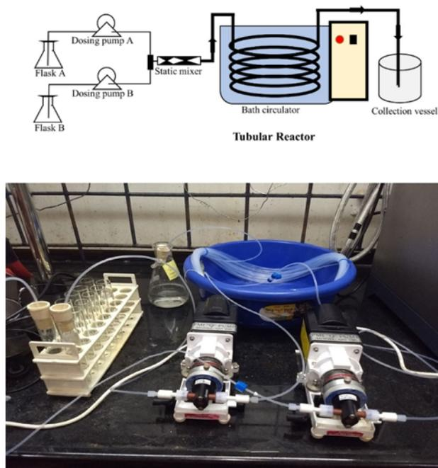
**Figure 2.** Schematic and actual image of the tubular reactor.
