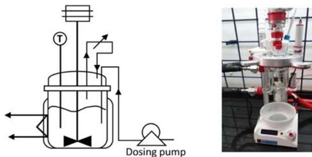
**Figure 1.** Schematic and actual image of the batch reactor.
