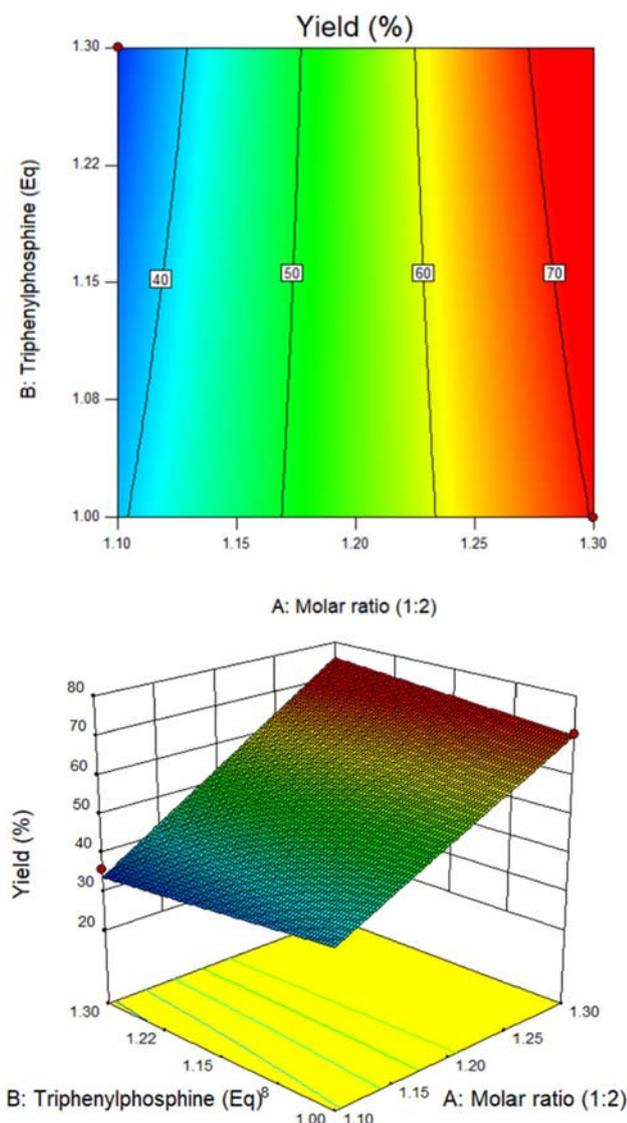
**Figure 3.** 1-(cyclohexyloxy)-2-methylbenzene (3) DoE analysis for the tubular reactor experiments (a) Contour plot and (b) Surface plot.
