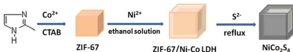
**Scheme 1.** Schematic diagram of NiCo<sub>2</sub>S<sub>4</sub> preparation process.
