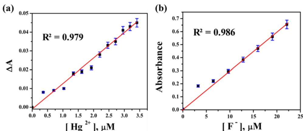
**Figure 3.** Calibration plot of **R** with (a)  $\text{Hg}^{2+}$  and (b)  $\text{F}^-$ .
