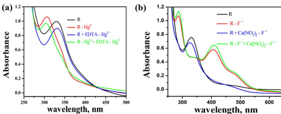
**Figure 6.** Reversible changes of **R** (20  $\mu\text{M}$ ) with (a)  $\text{Hg}^{2+}$  and EDTA (b)  $\text{F}^-$  and  $\text{Ca}(\text{NO}_3)_2$ .
