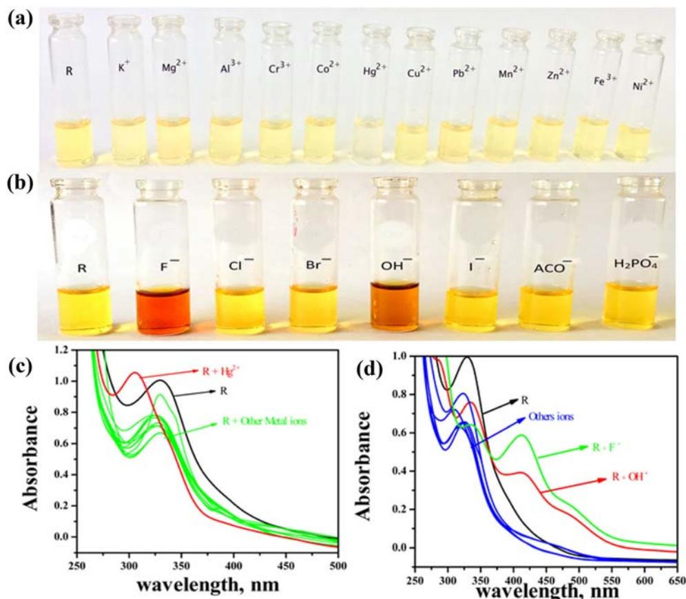
**Figure 1.** Colorimetric and UV-Visible spectral performance of **R** (20  $\mu$ M) with various selected analyte (2 mM): metal ions (a, c) and anions (b, d).
