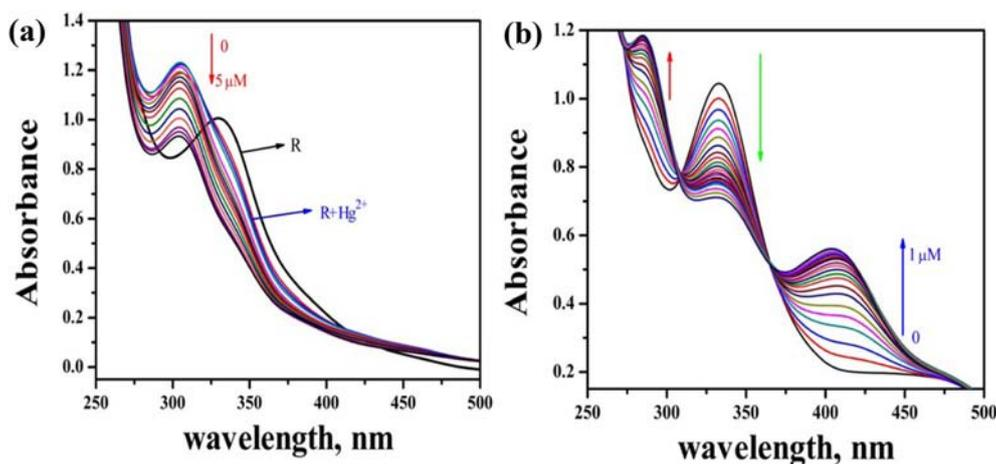
**Figure 2.** (a) UV–Visible spectral changes of **R** ( $2 \times 10^{-5}$  M) in aqueous media after the addition of  $\text{Hg}^{2+}$  (0–5  $\mu\text{M}$ ), (b)  $\text{F}^-$  (0–1  $\mu\text{M}$ ).
