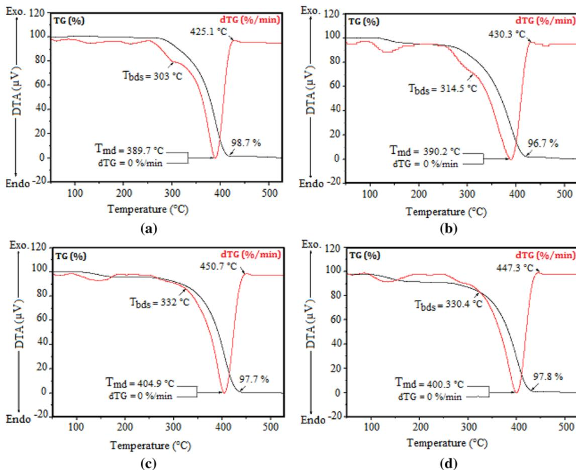
**Figure 9.** Curves of  $dTG$  ( $\% \cdot \text{min}^{-1}$ ) and  $TG$  (%) of pure Ps and Ps-P film catalysts. (a) Ps film  $F_0$ , (b) Ps-P film  $F_1$ , (c) Ps-P film  $F_2$ , and (d) Ps-P film  $F_3$ .  $T_{bds}$ , temperature of brutal degradation start;  $T_{md}$ , temperature of maximum degradation.
