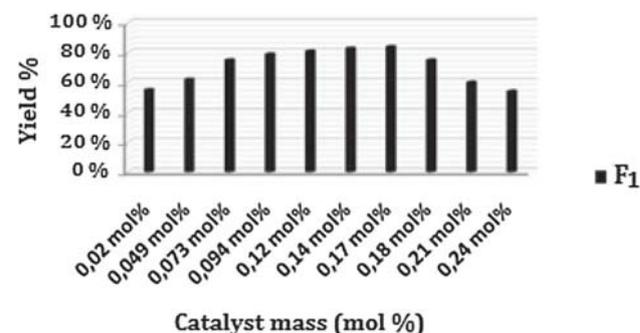
**Figure 10.** Effect of the F<sub>1</sub> film catalyst mass on the Knoevenagel reaction yield.
