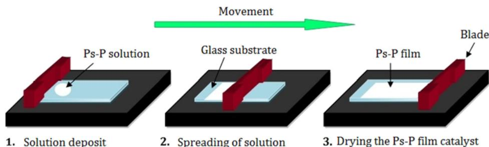
**Figure 1.** Synthesis of Ps-P film catalysts by doctor blade method.
