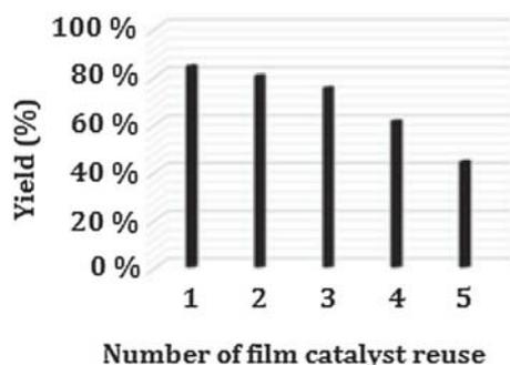
**Figure 11.** The reuse of  $F_1$  film catalyst in Knoevenagel condensation reaction.
