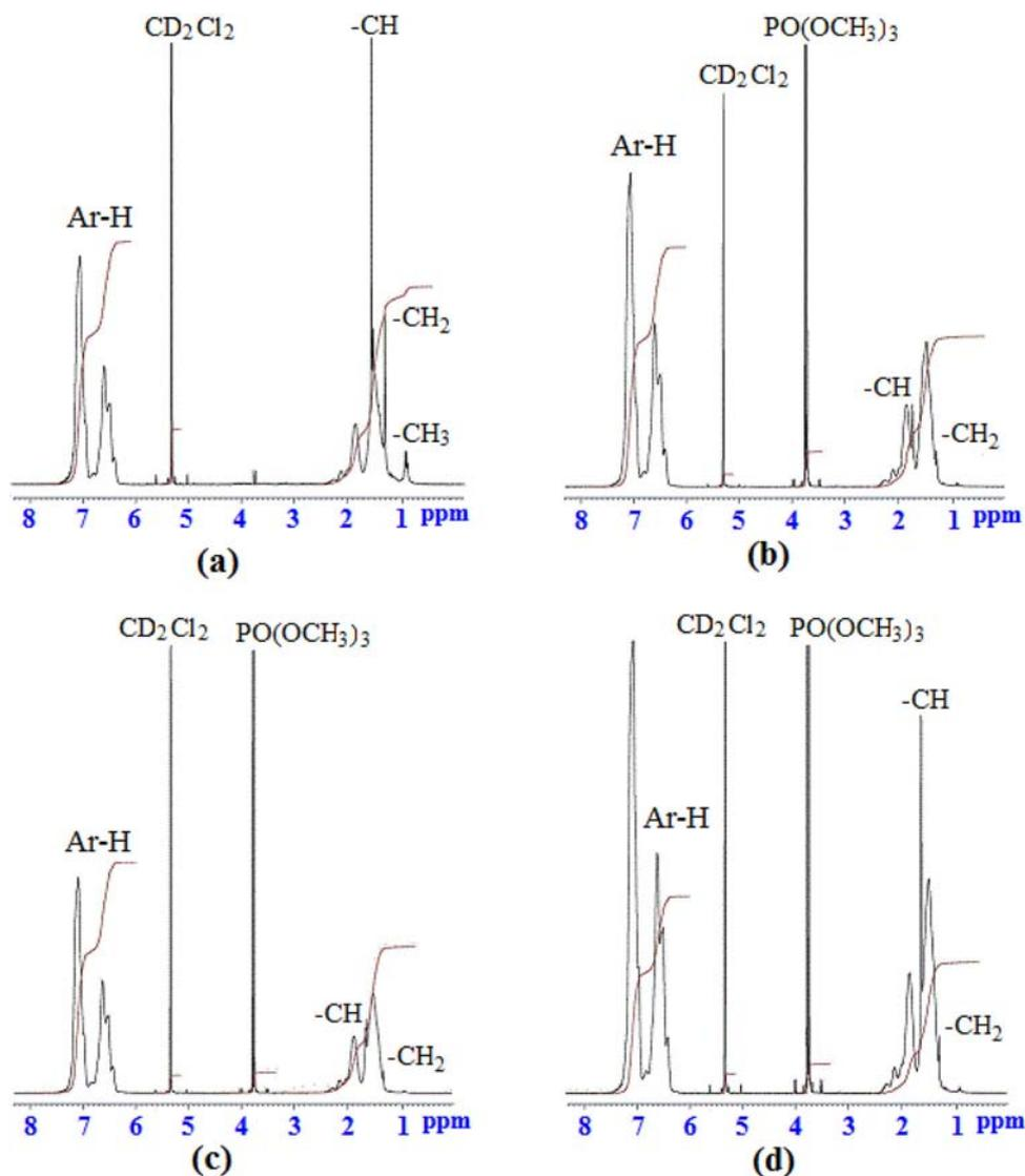
**Figure 3.**  $^1\text{H}$  NMR spectra of pure Ps film  $F_0$  (a) and Ps-P film catalysts  $F_1$  (b),  $F_2$  (c) and  $F_3$  (d).
