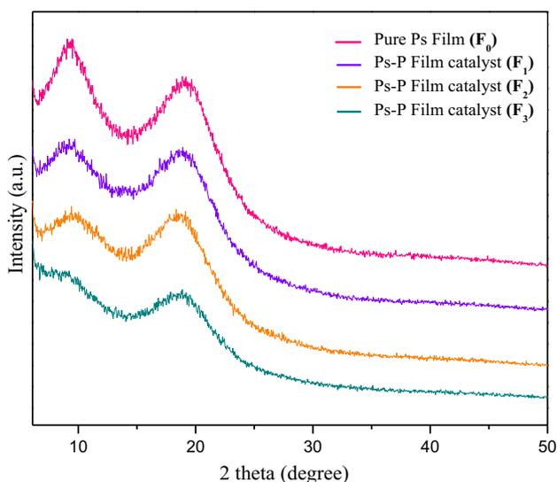
**Figure 8.** X-ray diffraction patterns of the Ps ( $F_0$ ) and Ps-P film catalysts ( $F_1$ ,  $F_2$ ) and ( $F_3$ ).
