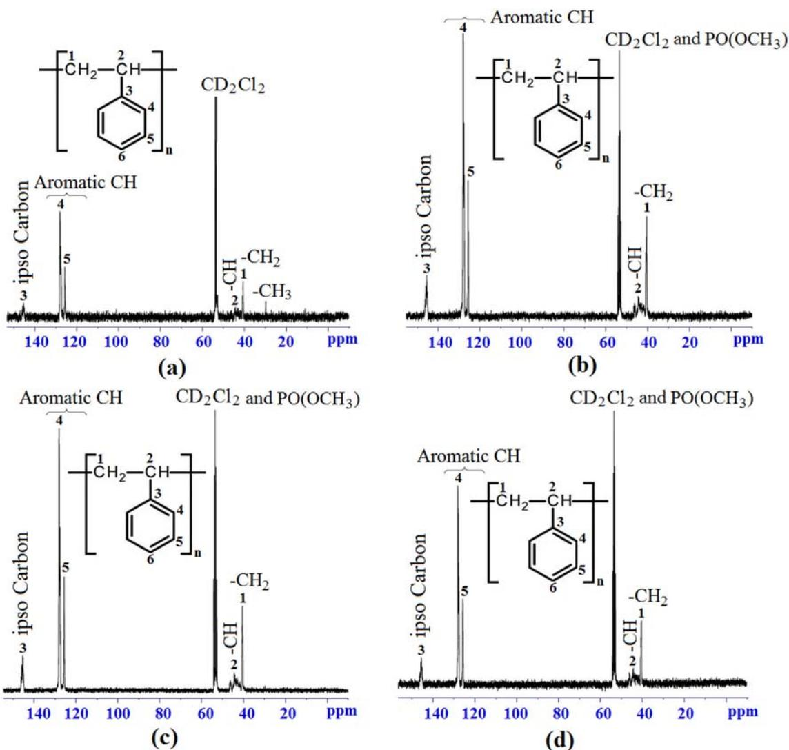
**Figure 4.**  $^{13}\text{C}$  NMR spectra of pure Ps film (a)  $F_0$  and Ps-P film catalysts (b)  $F_1$ , (c)  $F_2$  and (d)  $F_3$ .
