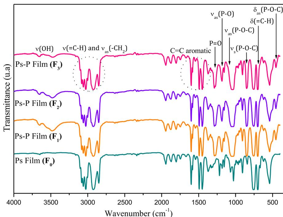
**Figure 2.** Infrared spectrum of the pure Ps ( $F_0$ ) and Ps-P film catalysts ( $F_1$ ,  $F_2$  and  $F_3$ ).
