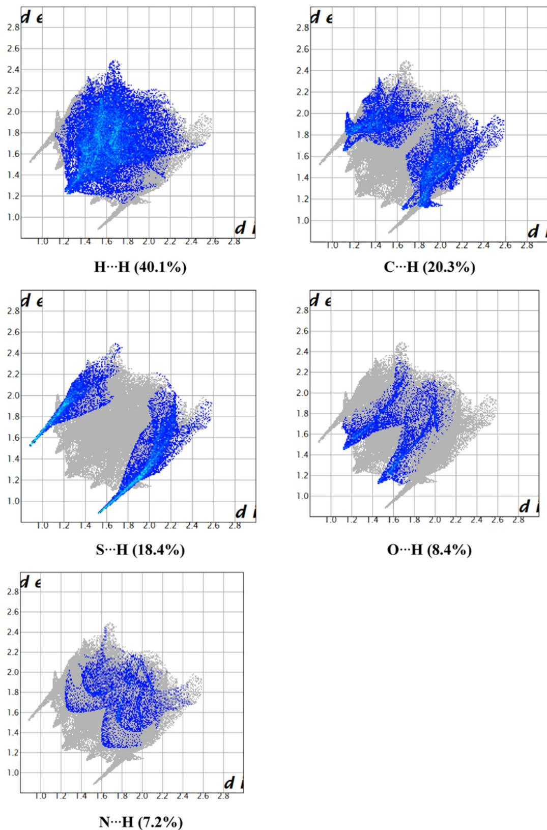
**Figure 4.** Relative contributions to the percentage of Hirshfeld surface area for the various intermolecular contacts in compound I.
