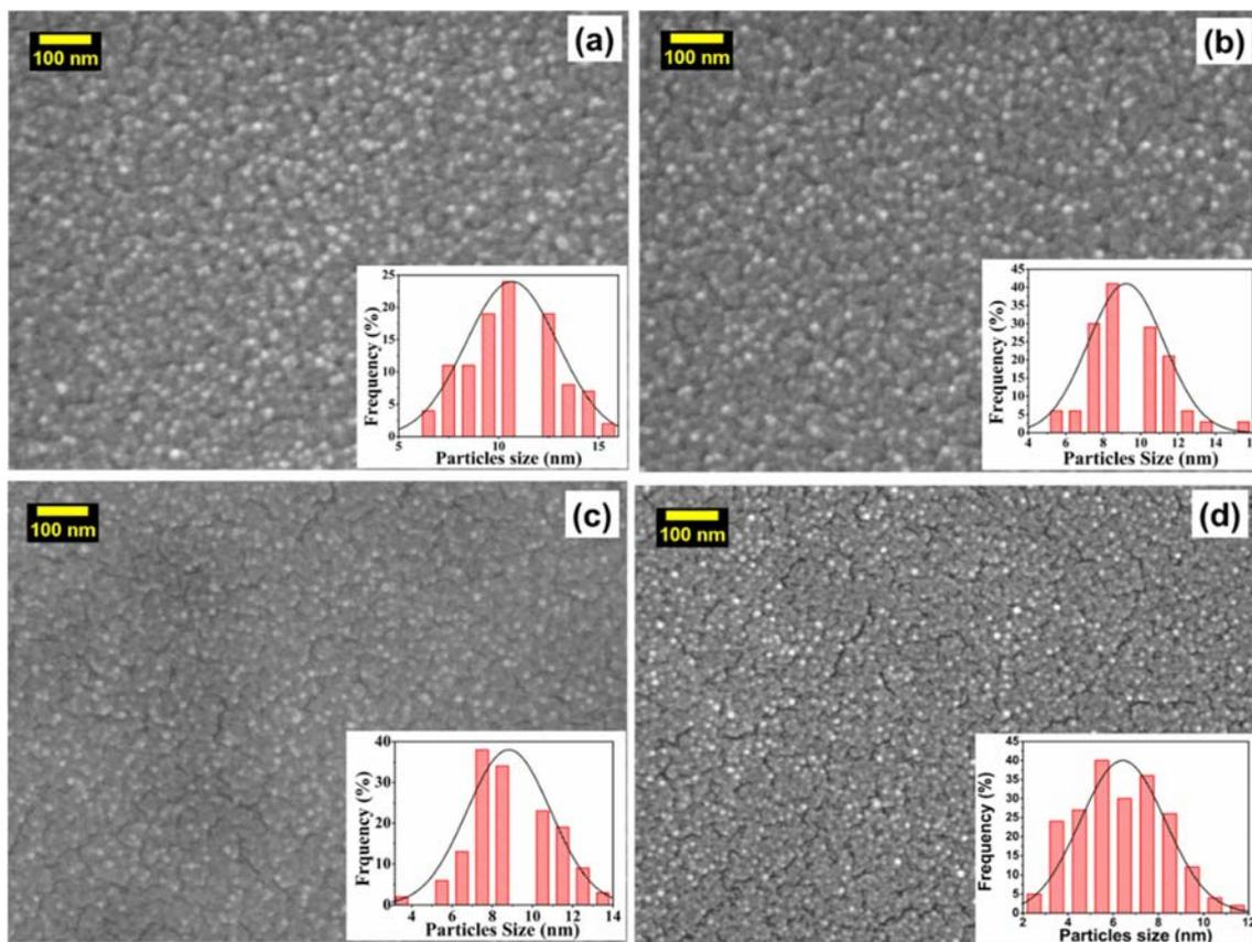
**Figure 3.** SEM image of silver nanoparticles supported PVA/PVP film at different PVA:PVP ratios (a) 100:0 (b) 95:05 (c) 90:10 (d) 85:15.
