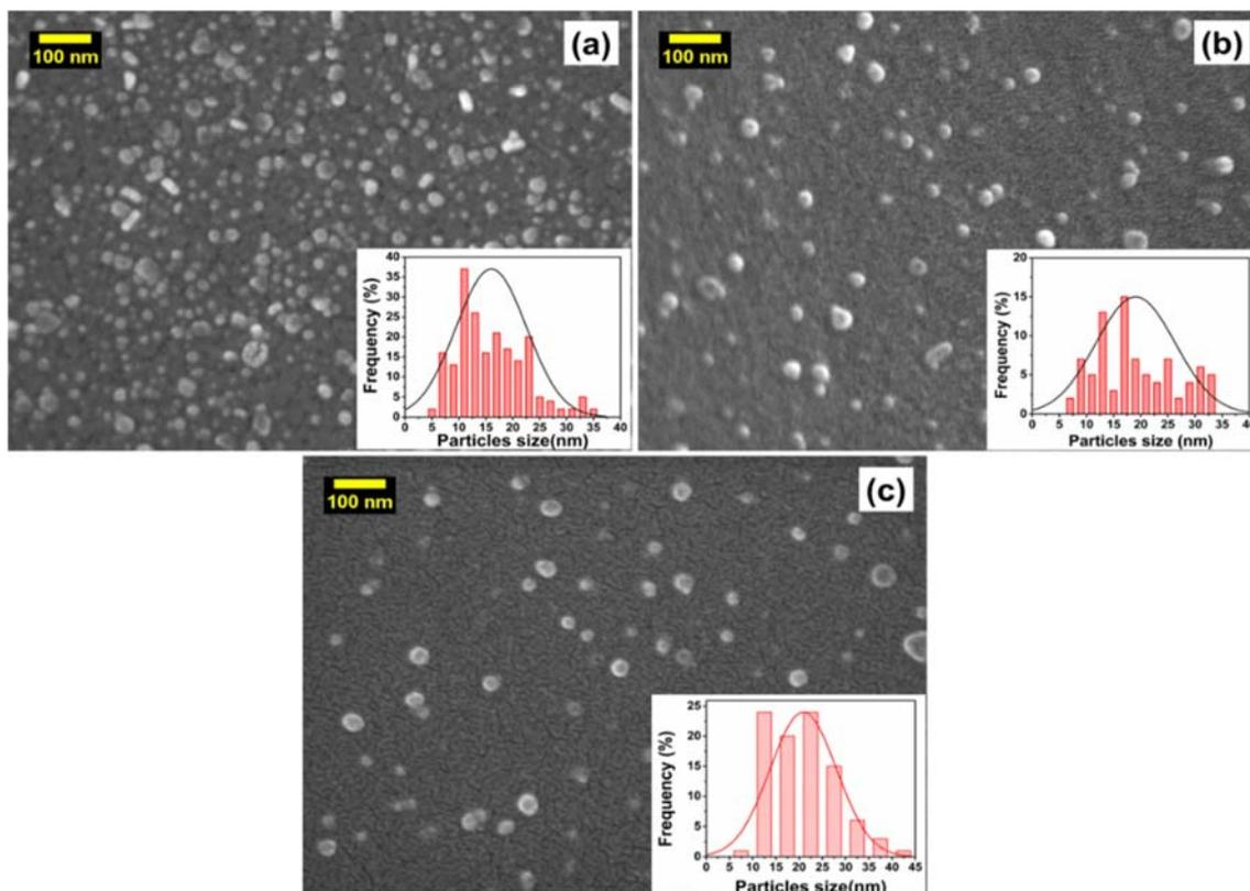
**Figure 9.** SEM image of catalyst film after (a) 1<sup>st</sup> run, (b) 3<sup>rd</sup> run, (c) 4<sup>th</sup> run.
