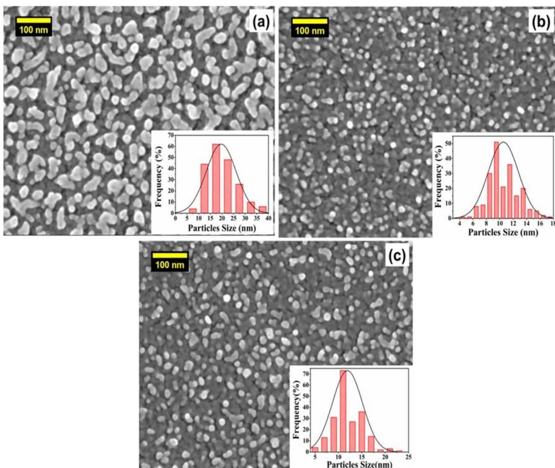
**Figure 2.** SEM images of Agnp supported PVA film at different microwave irradiation times (a) 6 min (b) 8 min (c) 10 min.
