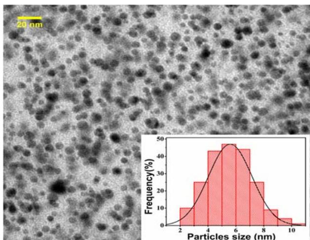
**Figure 4.** TEM image of silver nanoparticles supported PVA/PVP film at PVA:PVP (90:10) obtained at 8 min microwave irradiation time.
