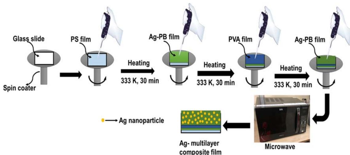
**Scheme 1.** Schematic diagram of synthesis process of Ag-nanoparticles supported multilayered composite film.
