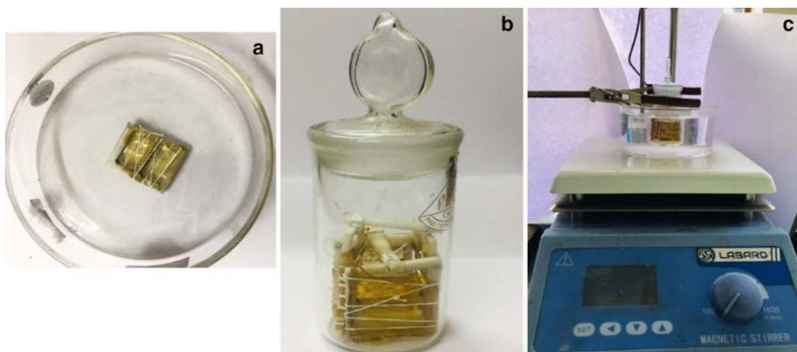
**Scheme 2.** Images of (a) film wrapped in teflon frame, (b) reaction vial with catalyst films, (c) overall experimental setup.
