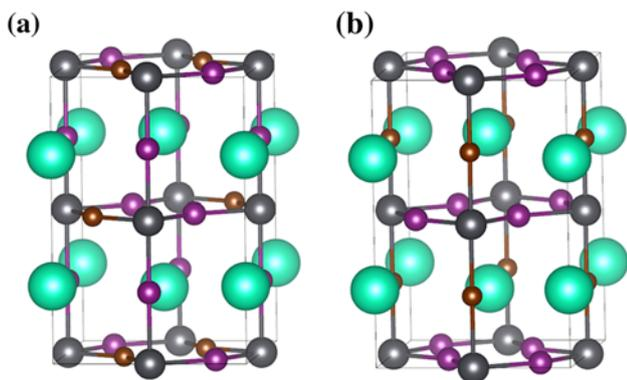
**Figure 1.** The crystal structure of CsPbI<sub>2</sub>Br suggested by ref. 40 (a) and ref. 45 (b). The green, gray, purple and brown balls denote Cs, Pb, I and Br atoms respectively.
