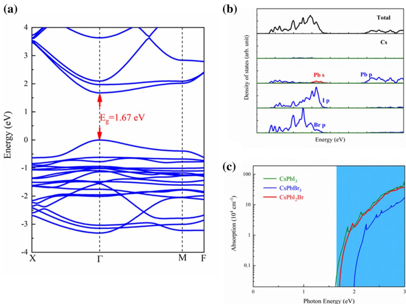
**Figure 2.** The PBE calculated (a) band structure, (b) projected density of states and (c) light absorption. The VBM energy in (a) and (b) is aligned to the zero energy. The blue region in the absorption curve (c) denotes the visible light range.
