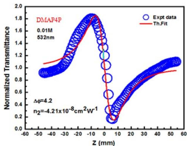
**Figure 7.** Nonlinear refraction curve **DMAP4P**. Solid line is a fit of data to Eq. (2) with  $\Delta = 4.2$ .
