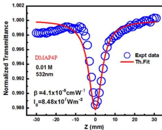
**Figure 6.** Open aperture curve for **DMAP4P**. Solid line is fitted to Eq. (1), with  $\beta_{\text{eff}} = 4.1 \times 10^{-5}$  cm/W.
