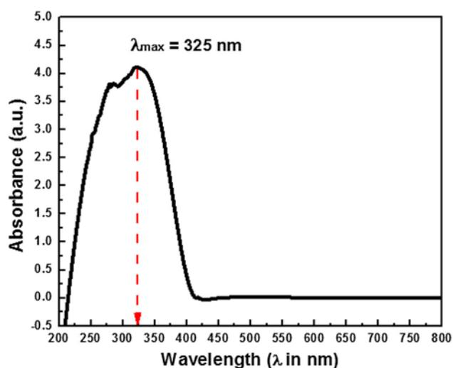
**Figure 4.** UV-Visible Spectrum of **DMAP4P**.
