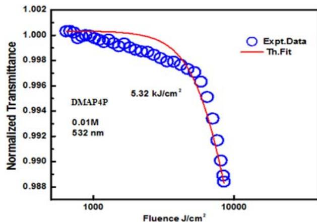
**Figure 8.** Optical limiting behavior of **DMAP4P**.
