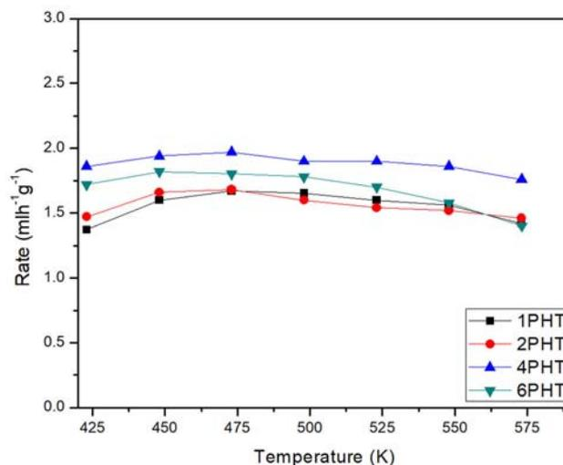
**Figure 6.** A plot of rate variation with temperature on 1–6wt% Pd/HT catalysts.
