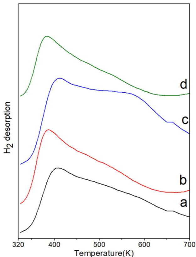
**Figure 4.** H<sub>2</sub>-TPD patterns of 1–6wt% Pd/HT catalysts (a) 1PHT, (b) 2PHT, (c) 4PHT and (d) 6PHT.
