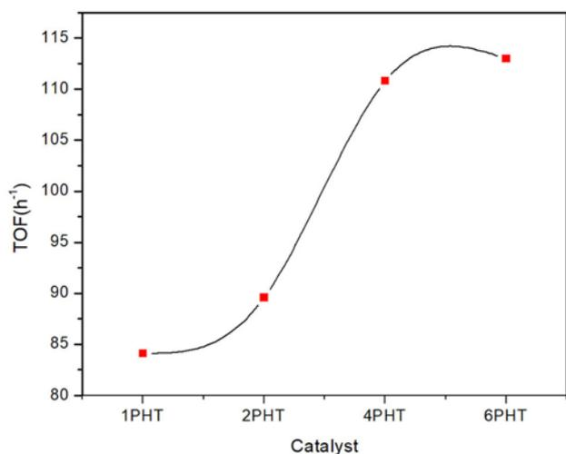
**Figure 8.** Variation of TOF with 1–6wt% Pd/HT catalysts.
