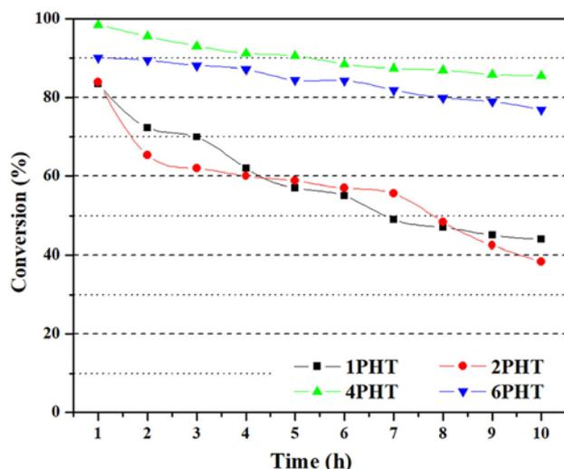
**Figure 7.** Time on stream patterns of 1–6wt% Pd/HT catalysts at 473 K.
