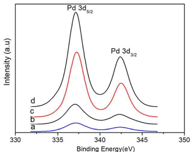
**Figure 3.** Pd 3d XPS spectra of calcined catalysts (a) 1PHT, (b) 2PHT, (c) 4PHT and (d) 6PHT.
