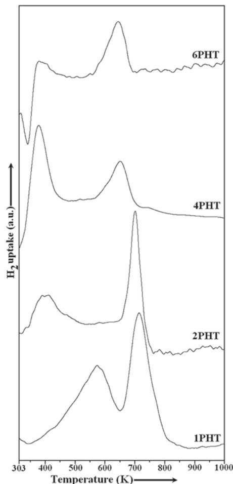
**Figure 5.** TPR patterns of 1–6wt% Pd/HT catalysts.
