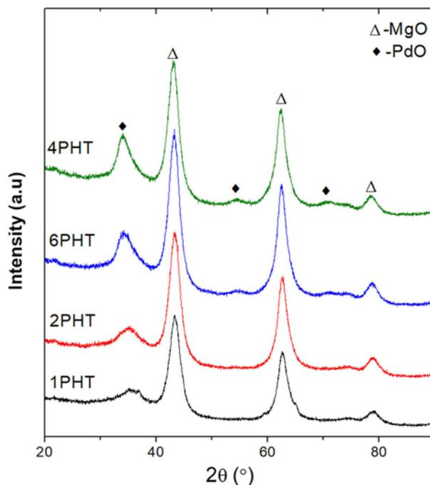
**Figure 2.** X-ray diffraction patterns of calcined 1–6wt% Pd/HT catalysts.
