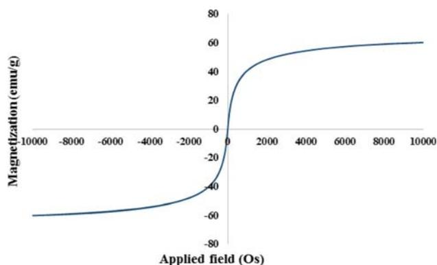
**Figure 3.** Hysteresis loops of  $\text{Fe}_3\text{O}_4$ @Diphenyl phosphate creatine.
