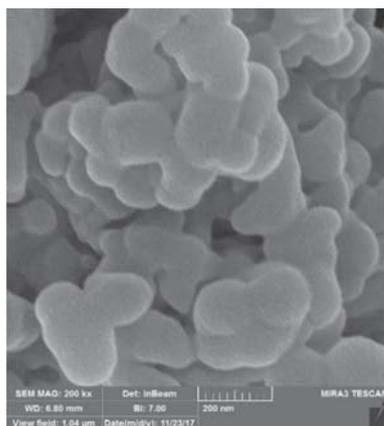
**Figure 2.** FE-SEM micrographs of  $\text{Fe}_3\text{O}_4$ @Diphenyl phosphate creatine.
