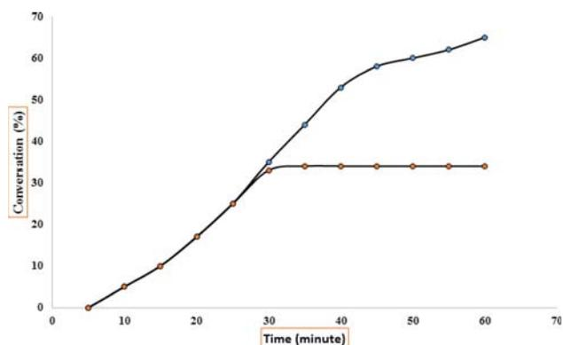
**Figure 8.** Leaching test for catalyst during a catalytic reaction.
