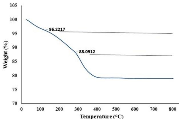
**Figure 5.** TGA of  $\text{Fe}_3\text{O}_4$ @Diphenyl phosphate creatine.
