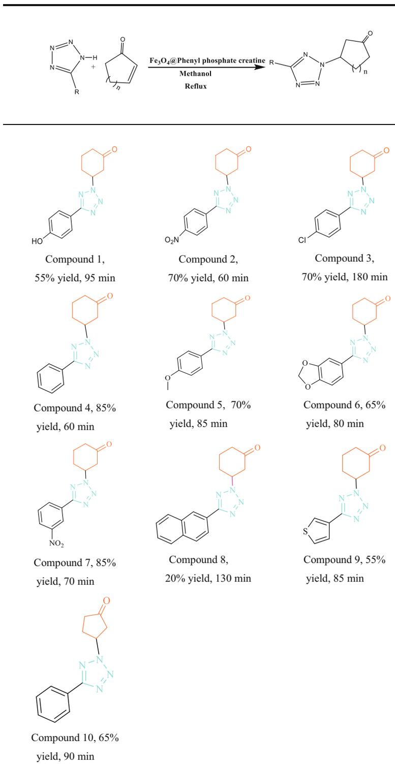
Reaction conditions: 5-substituted tetrazole derivatives (2 mmol) and  $\alpha$ ,  $\beta$ -unsaturated carbonyl (2 mmol) in methanol (10 mL) and the catalyst (50 mg) at 65 °C.
