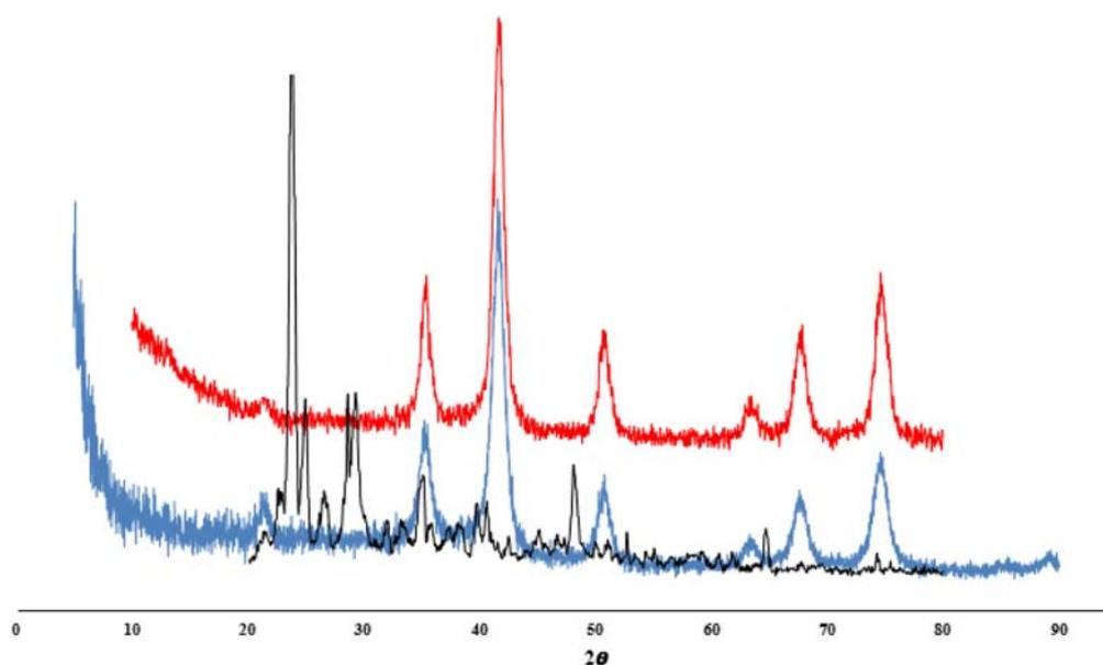
**Figure 4.** XRD patterns of Diphenyl phosphate creatine (Black curve),  $\text{Fe}_3\text{O}_4$  (Red curve) and  $\text{Fe}_3\text{O}_4$ @Diphenyl phosphate creatine (Blue curve).
