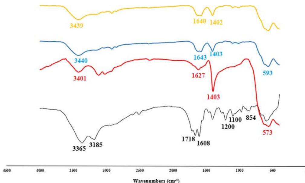
**Figure 1.** FT-IR spectra of Diphenyl phosphate creatine (black curve), Fe<sub>3</sub>O<sub>4</sub> (red curve) and Fe<sub>3</sub>O<sub>4</sub>@Diphenyl phosphate creatine before (blue curve) and after reaction (yellow curve).
