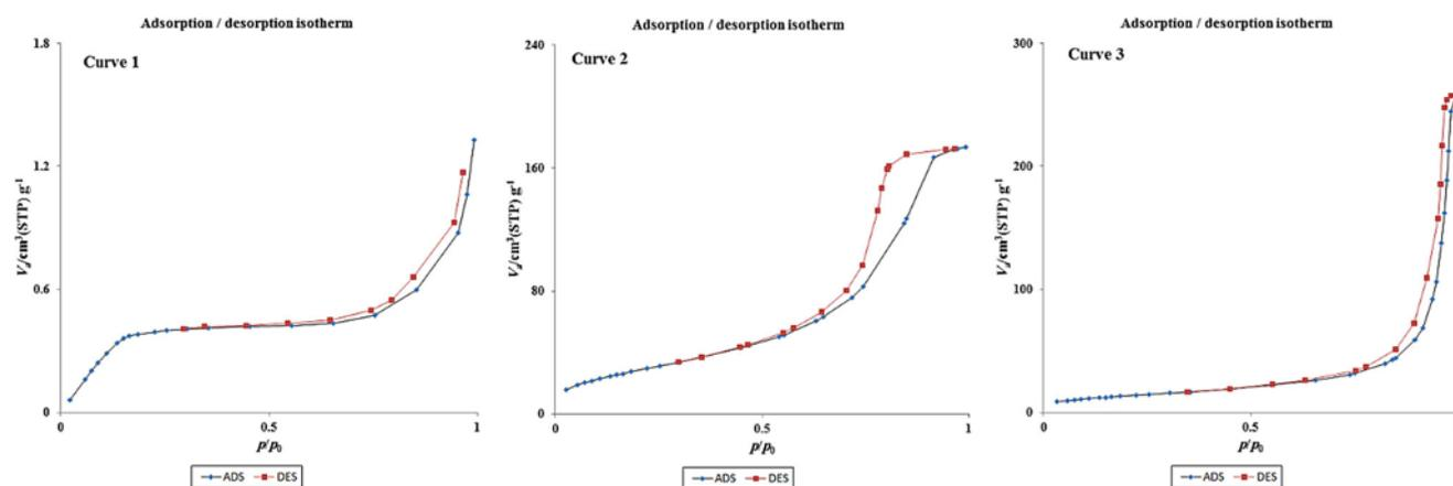
**Figure 6.** Nitrogen adsorption-desorption isotherms of Diphenyl phosphate creatine (curve 1),  $\text{Fe}_3\text{O}_4$  (curve 2) and  $\text{Fe}_3\text{O}_4$ @Diphenyl phosphate creatine (curve 3).
