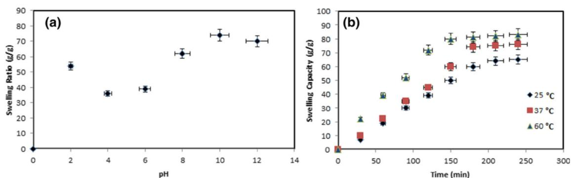
**Figure 2.** (a) Swelling kinetics of DCMC-cl-G hydrogel at different pH values and (b) swelling capacity of DCMC-cl-G hydrogel with temperature and time.
