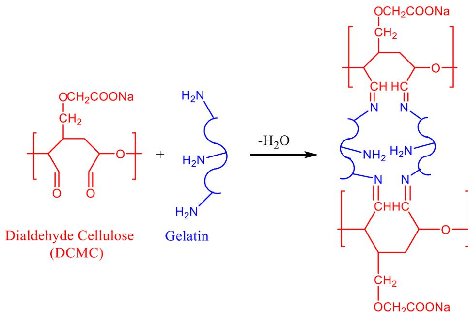
**Scheme 1.** Synthesis of DCMC-cl-G from DCMC and Gelatin via the Schiff base reaction.
