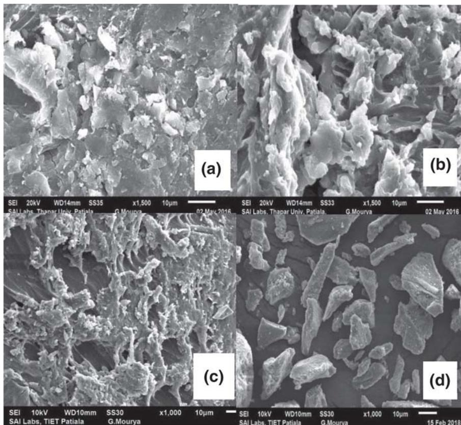
**Figure 10.** SEM images of DCMC-cl-G hydrogel during (a) 1<sup>st</sup> week, (b) 4<sup>th</sup> week, (c) 8<sup>th</sup> week, (d) 12<sup>th</sup> week of degradation.
