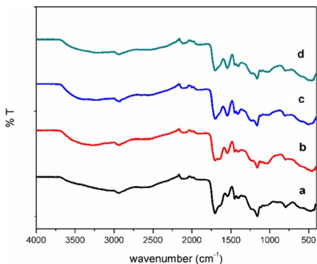
**Figure 11.** FTIR spectra of (a) DCMC-cl-G before degradation. (b) DCMC-cl-G after one-week degradation. (c) DCMC-cl-G after six weeks degradation. (d) DCMC-cl-G after twelve weeks degradation.
