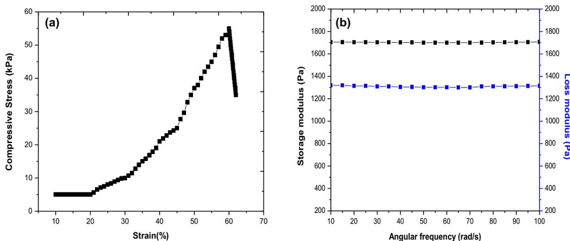
**Figure 4.** (a) Compressive strength of DCMC-cl-G hydrogel and (b) Storage modulus and loss modulus of the gel at a constant strain (1%).
