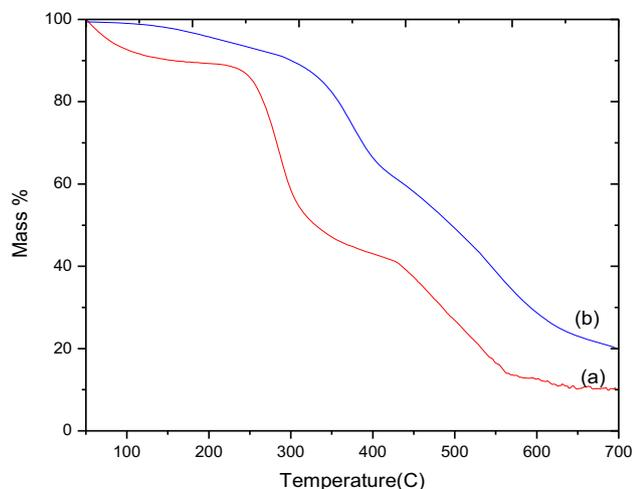
**Figure 5.** Thermograms of (a) DCMC and (b) DCMC-cl-G.
