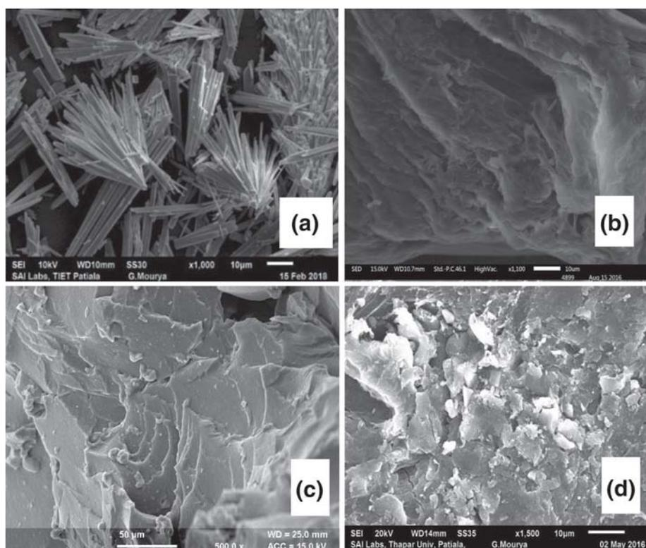
**Figure 3.** SEM images of (a) DCMC; (b) Gelatin; (c) and (d) DCMC-cl-G hydrogel.
