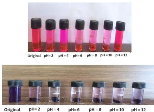
**Figure 6.** Effect of pH on RhB (top) and MV (bottom) dye adsorption by DCMC-cl-G at different pH values.
