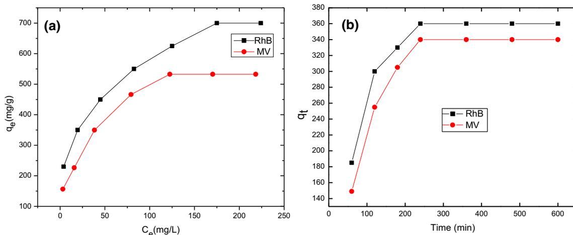
**Figure 8.** (a) Adsorption isotherms of RhB and MV dyes at 30 °C and pH 6.0 and (b) Effect of time and initial concentration of dyes on the adsorption of RhB and MV.
