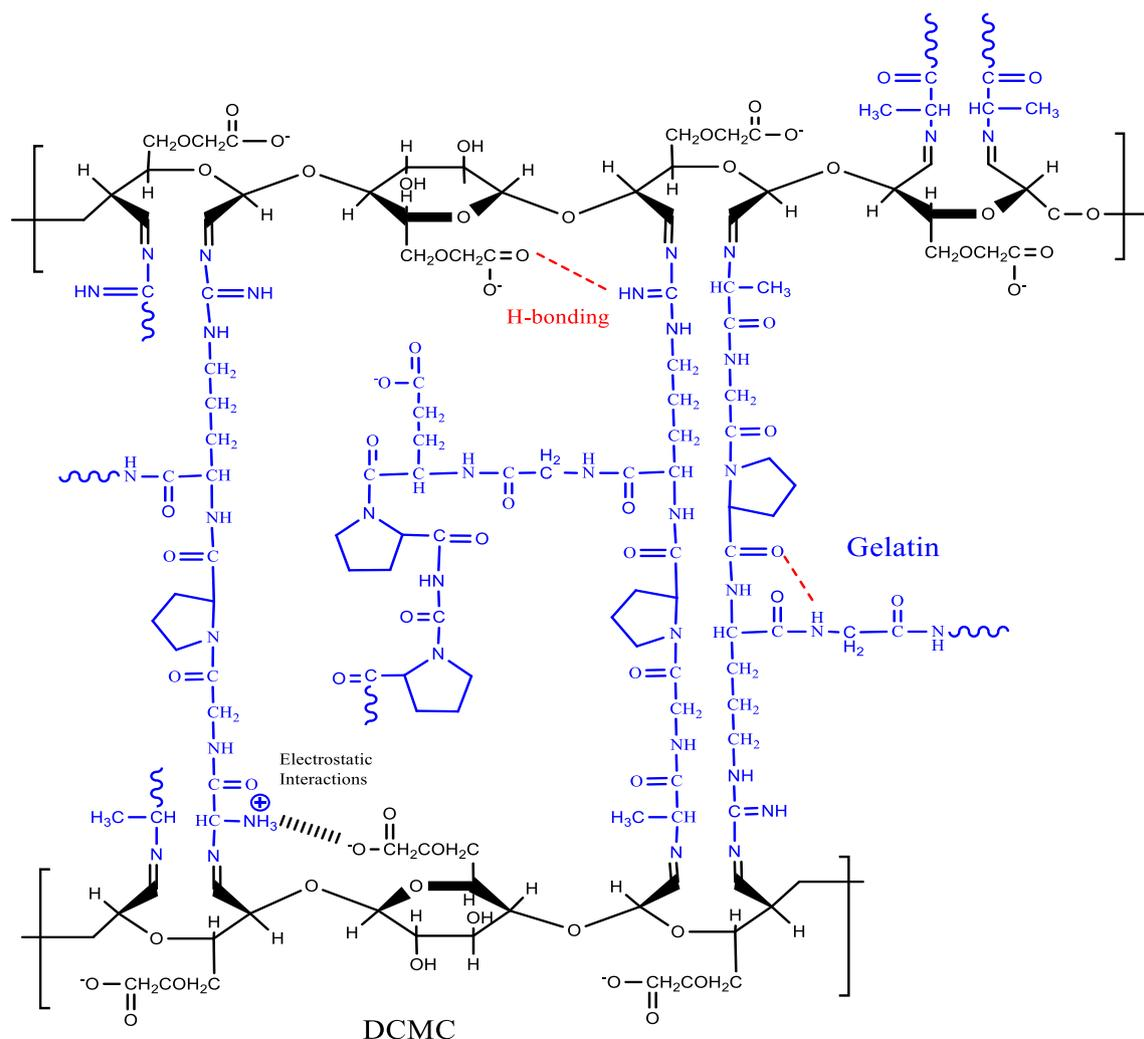
**Figure 1.** Schematic diagram of a cross-linked DCMC-cl-G hydrogel.
