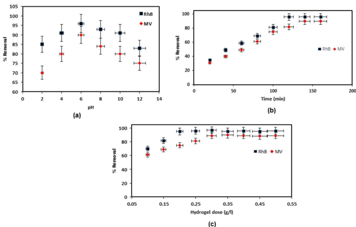
**Figure 7.** (a) Percentage removal of RhB and MV dyes, (b) effect of contact time on adsorption of RhB and MV at pH 6 and (c) effect of hydrogel dose on adsorption of RhB and MV.
