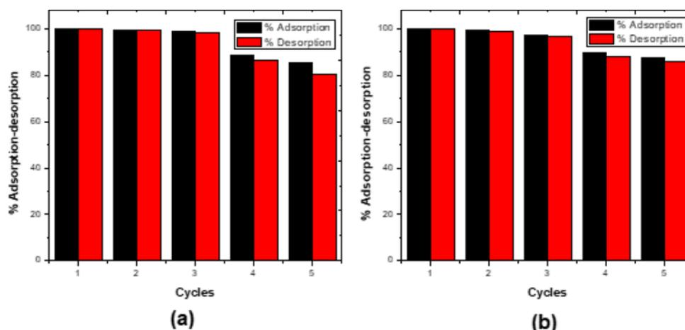
**Figure 9.** Performance of hydrogel for five cycles of adsorption-regeneration for (a) RhB and (b) MV.
