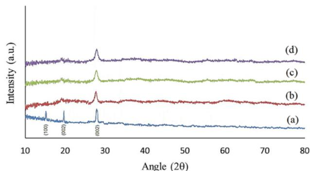
**Figure 1.** XRD patterns of (a) g-C<sub>3</sub>N<sub>4</sub>/rGO, (b) Co/g-C<sub>3</sub>N<sub>4</sub>/rGO, (c) Ni/g-C<sub>3</sub>N<sub>4</sub>/rGO, (d) Co<sub>2</sub>Ni1/g-C<sub>3</sub>N<sub>4</sub>/rGO.
