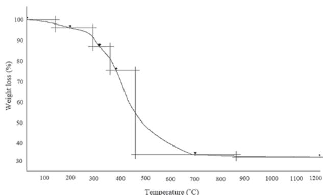
**Figure 4.** TGA curve of Co<sub>2</sub>Ni<sub>1</sub>/g-C<sub>3</sub>N<sub>4</sub>/rGO.
