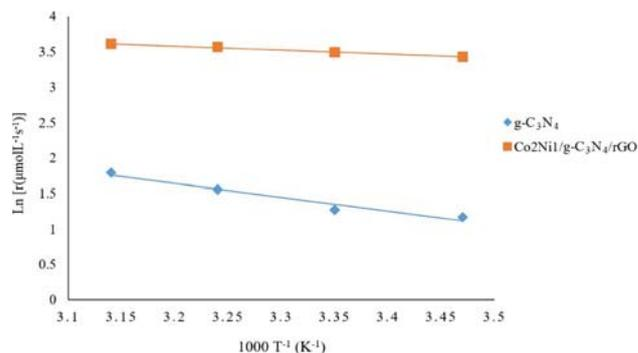
**Figure 9.** Arrhenius plot of O<sub>2</sub> evolution rate ln(r) vs. 1/T over g-C<sub>3</sub>N<sub>4</sub> and Co<sub>2</sub>Ni1/g-C<sub>3</sub>N<sub>4</sub>/rGO.
