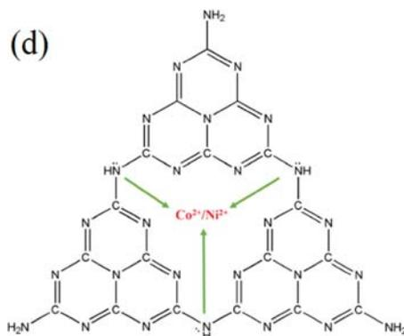
**Figure 5.** FE-SEM images of (a) g-C<sub>3</sub>N<sub>4</sub>, (b) g-C<sub>3</sub>N<sub>4</sub>/rGO, (c) Co<sub>2</sub>Ni<sub>1</sub>/g-C<sub>3</sub>N<sub>4</sub>/rGO, (d) schematic illustration of Co and Ni coordination to g-C<sub>3</sub>N<sub>4</sub>.
