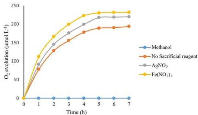
**Figure 8.** Effect of sacrificial reagents on O<sub>2</sub> evolution (1.75 g Fe(NO<sub>3</sub>)<sub>3</sub> or 10 mL methanol or 2.0 g AgNO<sub>3</sub>) 0.20 g Co<sub>2</sub>Ni1/g-C<sub>3</sub>N<sub>4</sub>/rGO at 7 h.
