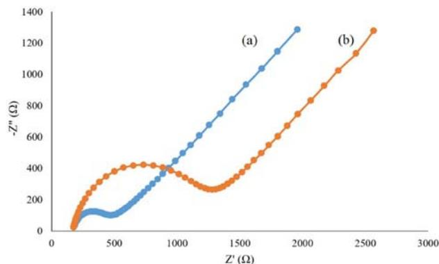
**Figure 7.** Electrochemical impedance spectroscopy (EIS) curves of (a) g-C<sub>3</sub>N<sub>4</sub>, (b) Co<sub>2</sub>Ni<sub>1</sub>/g-C<sub>3</sub>N<sub>4</sub>/rGO.
