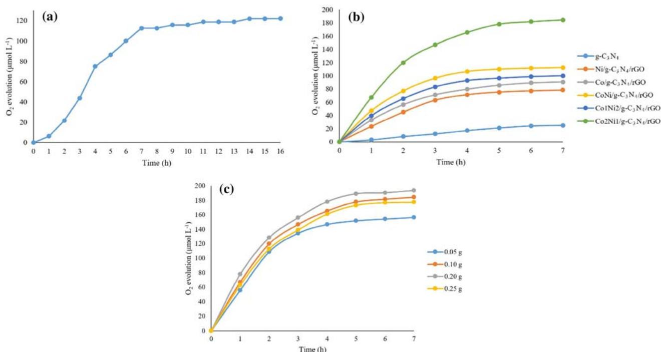
**Figure 6.** (a) Effect of reaction time (0.10 g of CoNi/ $g-C_3N_4$ /rGO), (b) effect of co-catalysts (0.10 g of photocatalyst at 7 h), (c) effect of catalyst weight (Co2Ni1/ $g-C_3N_4$ /rGO at 7 h).
