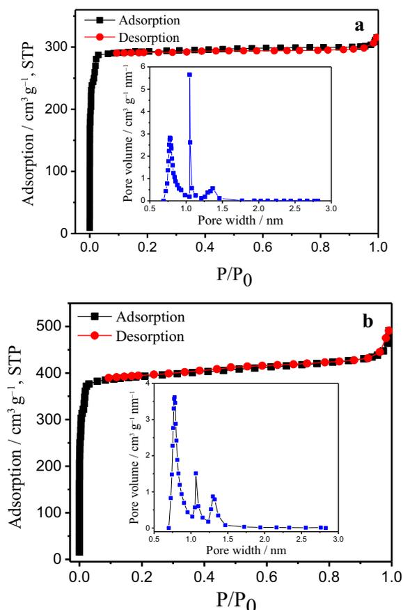
**Figure 5.** Nitrogen adsorption-desorption isotherms of (a)  $\text{MnO}_2@\text{CS}$  and (b) NC. Insets show corresponding pore size distributions.
