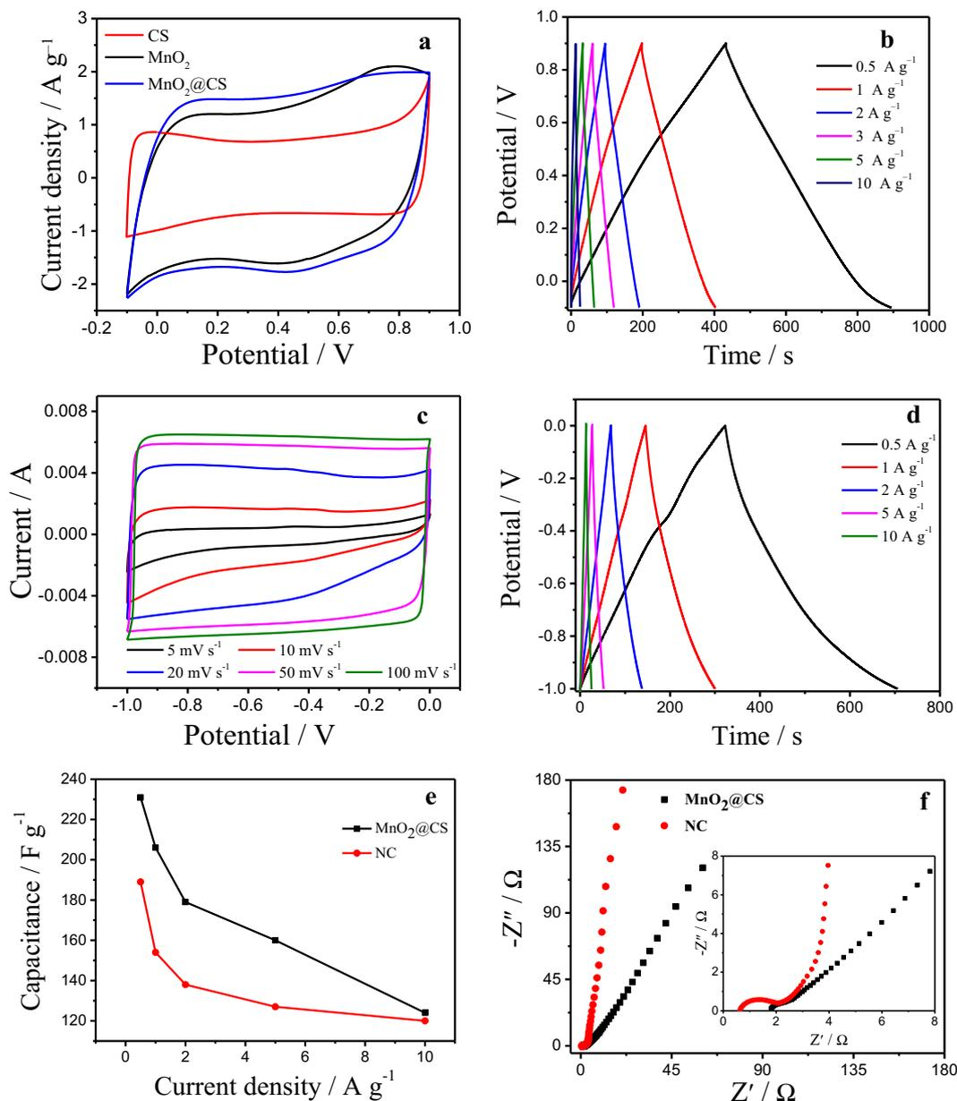
**Figure 6.** (a) Cyclic voltammograms of CS,  $\text{MnO}_2$ , and  $\text{MnO}_2@\text{CS}$  at a scanning rate of  $10 \text{ mV s}^{-1}$ . (b) Galvanostatic charge–discharge curves of  $\text{MnO}_2@\text{CS}$  for different current densities. (c) Cyclic voltammograms of NC at different scanning rates. (d) Galvanostatic charge–discharge curves of NC at different current densities. (e) Specific capacitance versus current density and (f) Nyquist plots of  $\text{MnO}_2@\text{CS}$  and NC.
