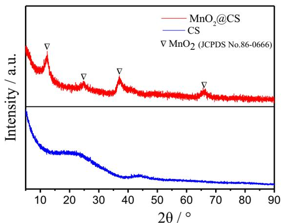
**Figure 3.** X-ray diffraction (XRD) patterns of the CS and  $\text{MnO}_2$ @CS samples.
