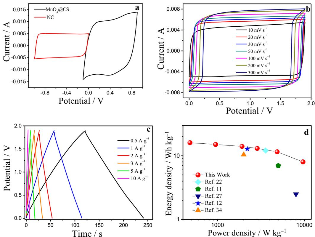
**Figure 7.** Cyclic voltammograms of (a) NC and MnO<sub>2</sub>@CS at 10 mV s<sup>-1</sup>; (b) MnO<sub>2</sub>@CS/NC asymmetric supercapacitor at different scanning rates. (c) Galvanostatic charge–discharge curves of the MnO<sub>2</sub>@CS/NC asymmetric supercapacitor at different current densities. (d) Ragone plot of MnO<sub>2</sub>@CS/NC device.
