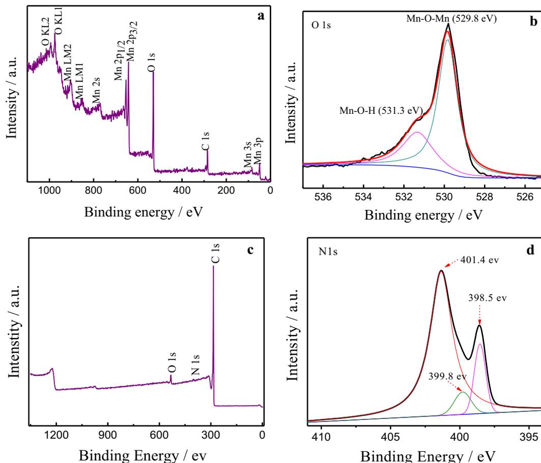
**Figure 4.** (a) X-ray photoelectron spectra (XPS) of the cathode material  $\text{MnO}_2$ @CS and (b) a close-up on the O1s peak. (c) XPS of the anode material NC and (d) a close-up on the N1s peak.
