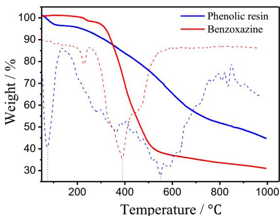
**Figure 1.** Thermal analysis curves for phenolic resin microspheres and benzoxazine. Solid and dashed lines represent thermogravimetric and differential thermogravimetric curves, respectively.
