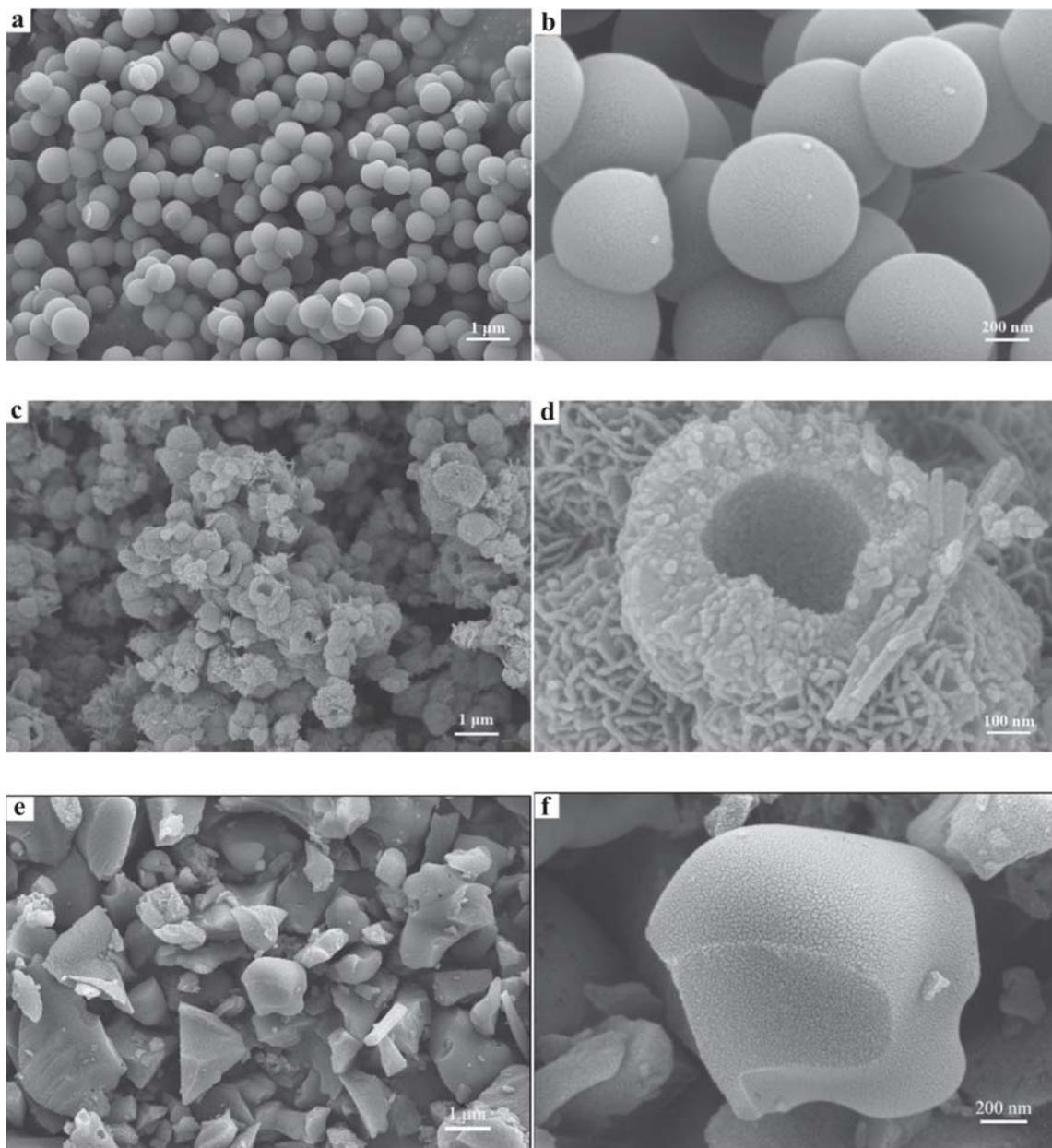
**Figure 2.** Scanning electron microscope (SEM) images of (a, b) carbon spheres after carbonization, (c, d)  $\text{MnO}_2$ @CS, and (e, f) NC.
