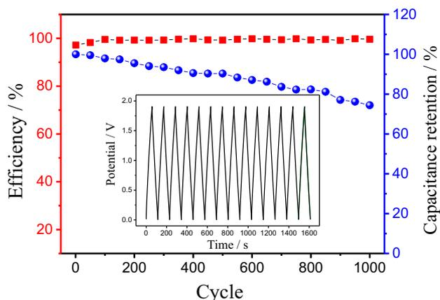
**Figure 8.** Charge–discharge efficiency and specific capacitance retention of the proposed MnO<sub>2</sub>@CS//NC asymmetric supercapacitor at a current density of 1 A g<sup>-1</sup>.
