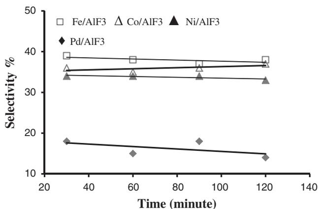
**Figure 4.** A plot of selectivity chlorosilane derivative ( $\text{Me}_3\text{SiCl}$ ) as a function of time for HDC process of  $\text{Me}_3\text{SiCHCl}_2$  over Pd, Ni, Fe and Co supported on  $\text{AlF}_3$  at  $200^\circ\text{C}$ .
