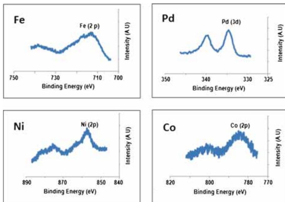
**Figure 1.** X-ray photoelectron spectra (XPS) for the prepared monometallic Pd, Fe, Co and Ni catalysts supported on AlF<sub>3</sub>.
