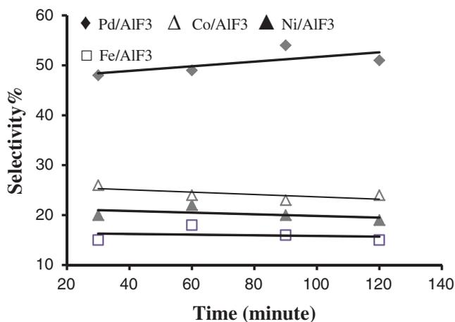
**Figure 3.** A plot of selectivity the monochloro product ( $\text{Me}_3\text{SiCH}_2\text{Cl}$ ) as a function of time for HDC process of  $\text{Me}_3\text{SiCHCl}_2$  over Pd, Ni, Fe and Co supported on  $\text{AlF}_3$  at  $200^\circ\text{C}$ .
