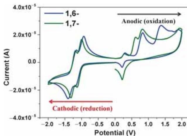
**Figure 7.** The cyclic voltammograms of **1** and **2** measured in dichloromethane solution (versus SCE) with ferrocenium/ferrocene as an internal standard, at 200 mV/s.
