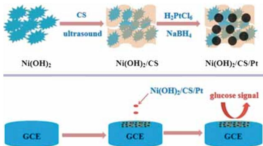
**Scheme 1.** Schematic illustration for the preparation of  $\text{Ni}(\text{OH})_2/\text{CS}/\text{Pt}/\text{GCE}$ .
