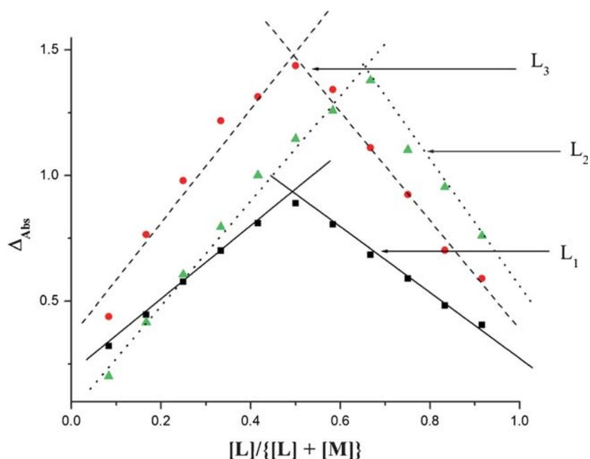
**Figure 4.** Typical Job's plots for the reaction between complex and ligands at pH = 7.4 and ionic strength = 0.1 mol dm<sup>-3</sup> NaClO<sub>4</sub>.
