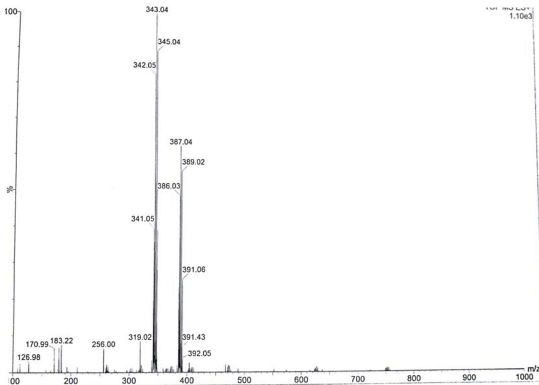
Figure 3. ESI Mass spectrum of the  $[Pd(2,2'\text{-bipyridine})(malonate)]$  complex.
