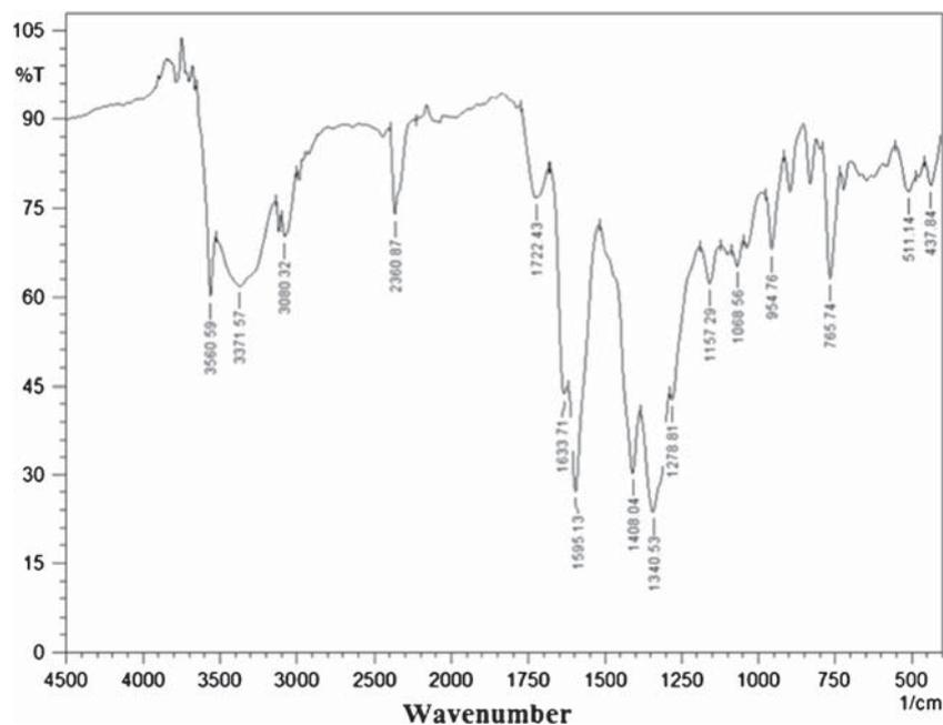
Figure 2. IR spectrum of the  $[Pd(2,2'\text{-bipyridine})(malonate)]$  complex.
