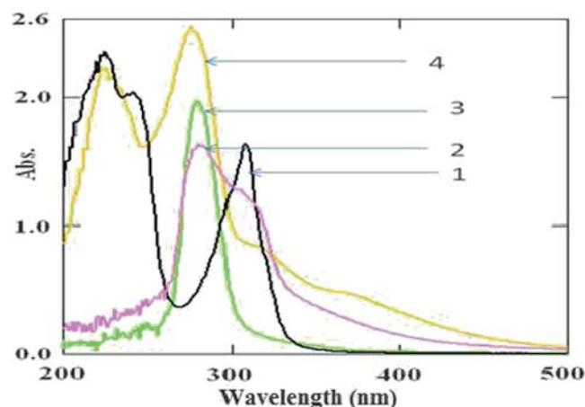
**Figure 1.** Absorption spectra of  $[Pd(2,2'\text{-bipyridine})(malonate)]$  complex (1), thioglycolic acid ( $L_1$ ) substituted product (2), thiourea ( $L_2$ ) substituted product (3) and thiosemicarbazide ( $L_3$ ) substituted product (4).  $[complex] = 2 \times 10^{-4}\text{ mol dm}^{-3}$ ,  $[ligand] = 4 \times 10^{-3}\text{ mol dm}^{-3}$ ,  $pH = 7.4$ , and quartz cell path length = 1 cm.
