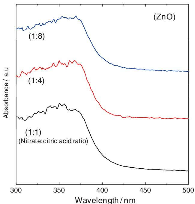
**Figure 6.** UV-Vis spectra of the samples obtained from representative N:C molar ratios (1:1, 1:4 and 1:8) of zinc nitrate and citric acid synthesized by modified sol-gel route.
