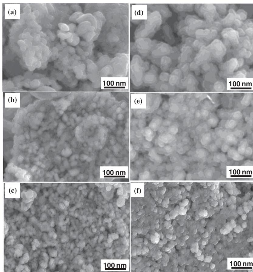
**Figure 7.** SEM images of surface of the samples from representative N/C ratios (a) (1:1), (b) (1:4) and (c) (1:8) of Cu system, and (d) (1:1), (e) (1:8) and (f) (1:8) of Zn system.
