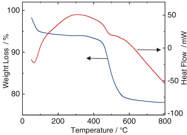
**Figure 2.** TGA/DTA curves recorded in air for the gel obtained from (1:8) NC ratio of copper nitrate and citric acid.
