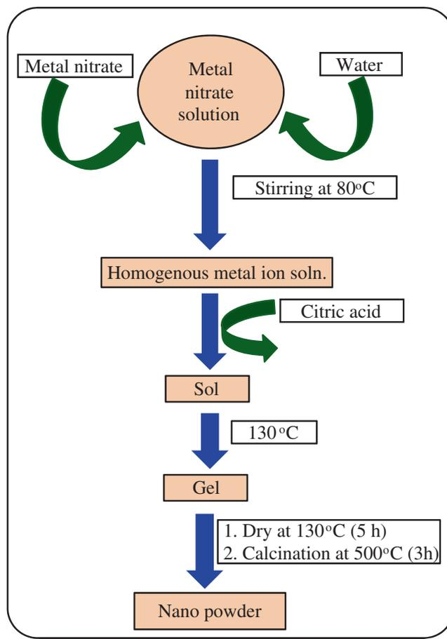
**Figure 1.** Schematic of the modified sol-gel process adopted in the present work.
