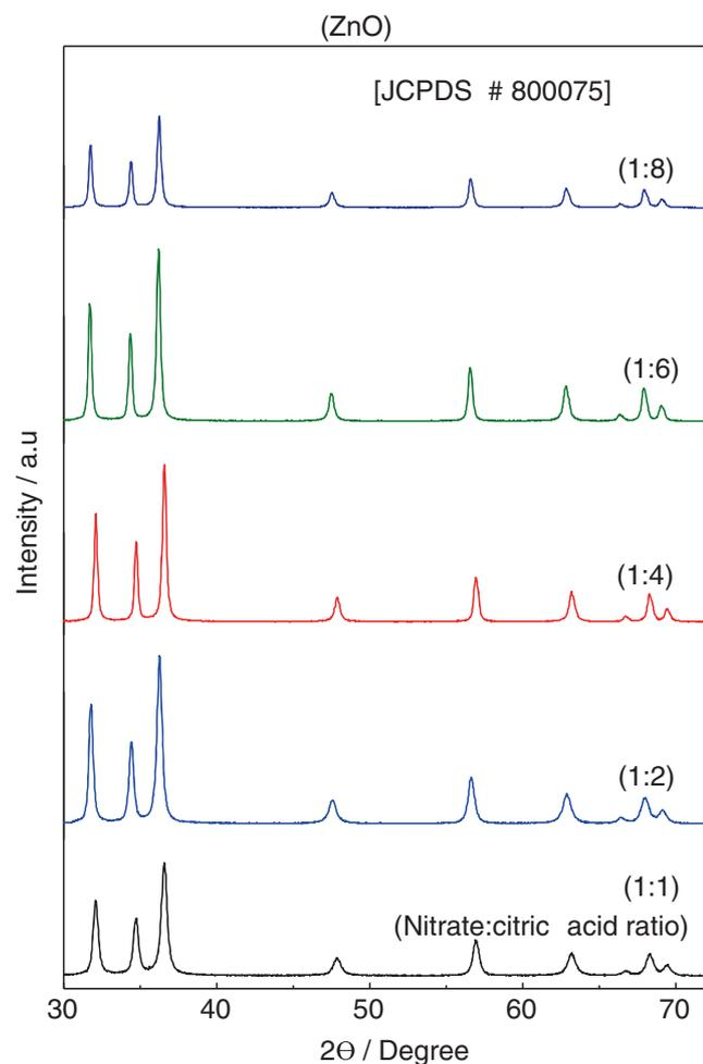
**Figure 4.** XRD patterns of the samples obtained from each of various N:C molar ratios (1:1-1:8) of zinc nitrate and citric acid.
