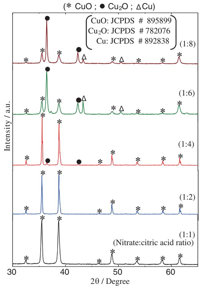
**Figure 3.** XRD patterns of the samples obtained from each of various N:C molar ratios (1:1-1:8) of copper nitrate and citric acid.
