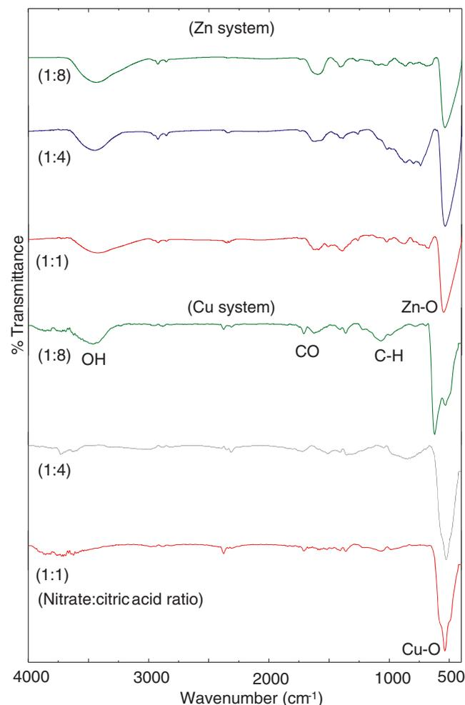
**Figure 5.** FT-IR spectra of the samples obtained from representative N:C molar ratios (1:1, 1:4 and 1:8) of metal nitrates and citric acid synthesized by modified sol-gel process.
