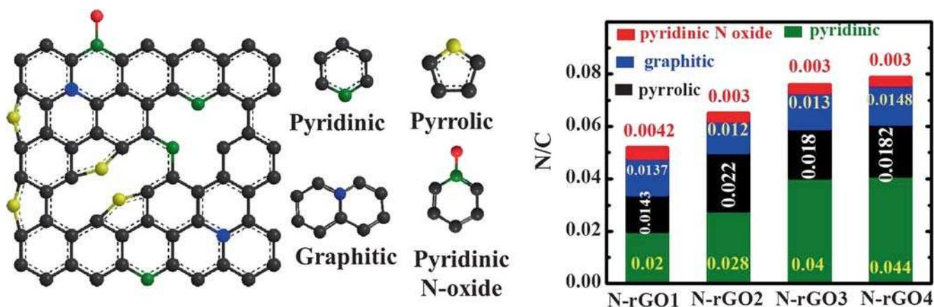
**Figure 4.** Four different types of nitrogen present in N-rGOs. The data given in the plot is the atomic ratio of the respective nitrogen and carbon (N/C) present in the samples.
