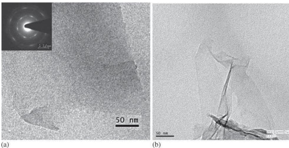
**Figure 2.** TEM image of N-rGO3 (a, b). The SAED pattern of the corresponding TEM image is shown in Figure 2a inset.
