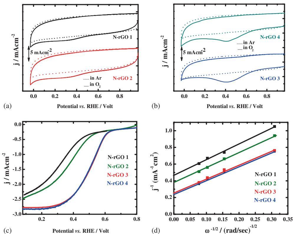
**Figure 5.** Cyclic voltammogram in Ar and O<sub>2</sub> saturated electrolyte presented by dotted and solid line, respectively, for (a) N-rGO1 and N-rGO2, (b) N-rGO3 and N-rGO4, scan rate 50 mV/s (c) Polarization curves for ORR on different N-rGO catalysts in 0.5 M H<sub>2</sub>SO<sub>4</sub> solution at 1600 rpm, scan rate, 5 mV/s. (d) corresponding Koutecky-Levich plot for the different N-rGOs at 0.27 V.
