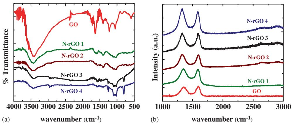
**Figure 1.** (a) FTIR and (b) Raman spectral profiles of GO and different N-rGOs.
