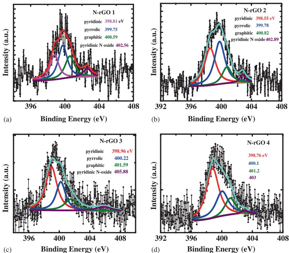
**Figure 3.** Deconvoluted XPS N1s spectral profiles of different N-rGOs.
