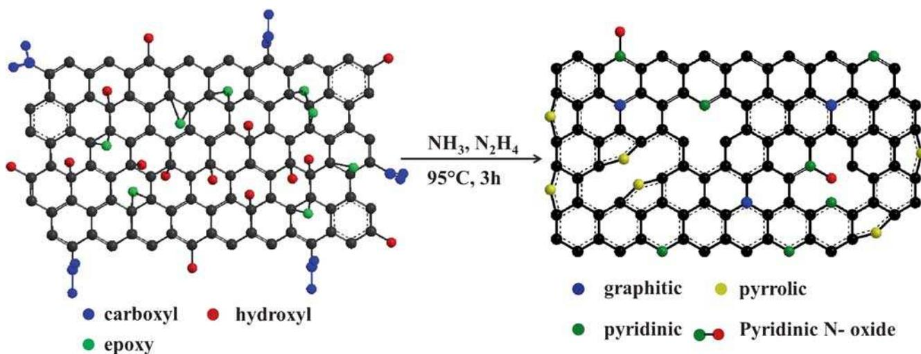
**Scheme 1.** Schematic illustration of the synthesis of N-rGO.
