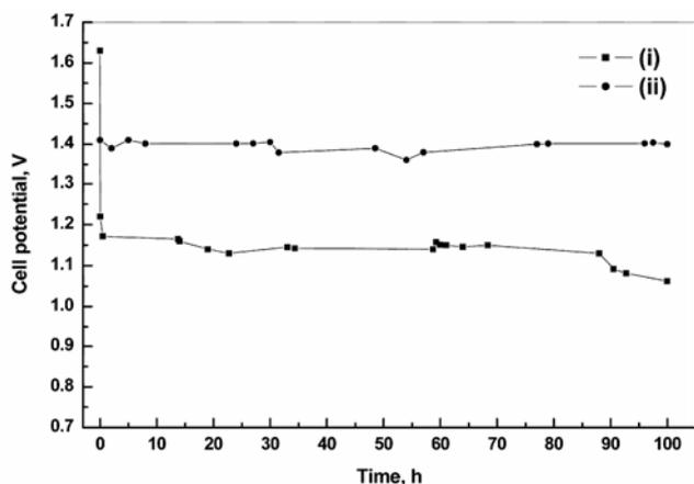
**Figure 6.** Data pertaining to cell performance durability tests on DBFCs with (i) polyvinyl alcohol hydrogel membrane, and (ii) Nafion<sup>®</sup>-117 membrane electrolytes.
