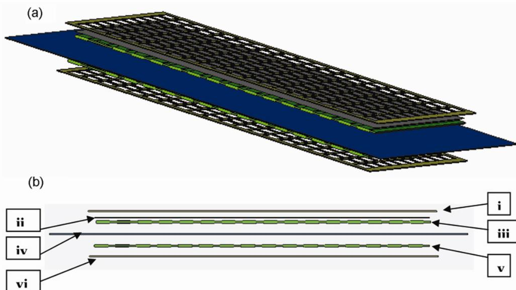
**Figure 1.** (a) Three-dimensional side-view of the MEA employing PHME; (b) two-dimensional side-view of the PHME-based MEA: (i) gold-plated SS mesh on anode side, (ii) anode catalyst layer, (iii) PVA + glutaraldehyde binder layer on anode side, (iv) PHME, (v) PVA + glutaraldehyde binder layer on cathode side, (vi) gold-plated SS mesh used as cathode.
