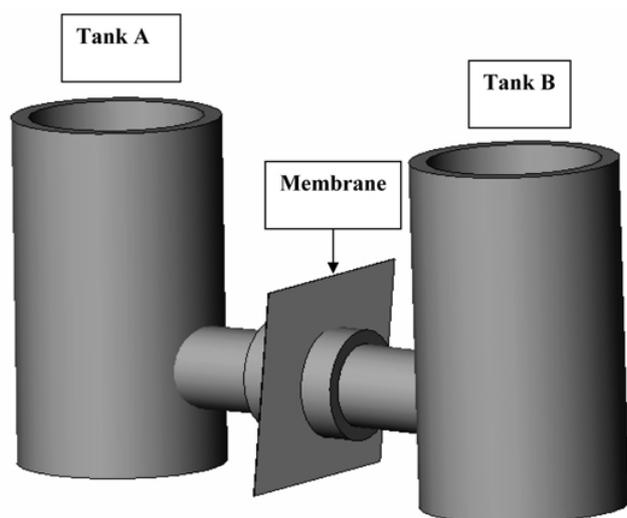
**Figure 3.** Schematic diagram of the set-up for *ex-situ* determination of extent of crossover of various chemical species employed in DBFCs through PHME and NME. 'Tank A' holds an aqueous solution of  $\text{H}_2\text{O}_2$ ,  $\text{NaBH}_4$ ,  $\text{H}_2\text{SO}_4$  or  $\text{NaOH}$  and 'Tank B' holds an equal volume of Millipore water.
