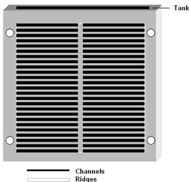
**Figure 2.** A schematic diagram of a typical fluid flow field plate machined from high-density graphite blocks with an active area of  $9 \text{ cm}^2$  that acted as storage tanks for fuel or oxidant.
