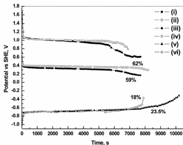
**Figure 5.** Chronopotentiometric data for determination of utilization efficiencies of NaBH<sub>4</sub> and H<sub>2</sub>O<sub>2</sub> in DBFCs: (i) cell potential data for PHME-based DBFC, (ii) cell potential data for NME-based DBFC, (iii) cathode potential data for PHME-based DBFC, (iv) cathode potential data for NME-based DBFC, (v) anode potential data for PHME-based DBFC, (vi) anode potential data for NME-based DBFC.
