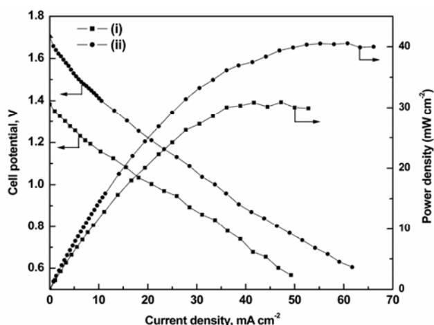
**Figure 4.** Cell performance data for DBFCs with (i) polyvinyl alcohol hydrogel membrane, and (ii) Nafion<sup>®</sup>-117 membrane electrolytes.
