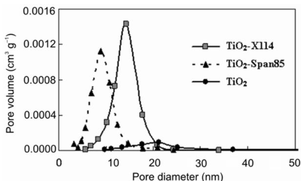
**Figure 3.** Pore size distributions of TiO<sub>2</sub>-X114, TiO<sub>2</sub>-Span85 and TiO<sub>2</sub> derived from desorption branches of N<sub>2</sub> adsorption/desorption isotherms.
