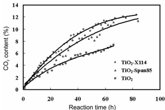
**Figure 7.** Photocatalytic performances of  $\text{TiO}_2$ -X114,  $\text{TiO}_2$ -Span85 and  $\text{TiO}_2$ .
