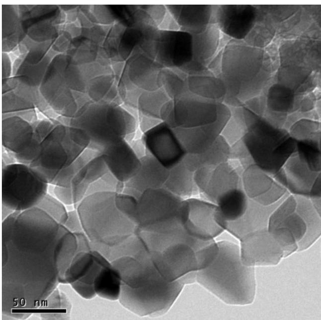
**Figure 4.** TEM image of sample TiO<sub>2</sub>-X114.
