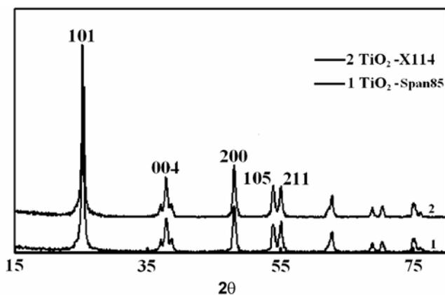
Figure 1. X-ray patterns of sample TiO<sub>2</sub>-X114 and TiO<sub>2</sub>-Span85.
