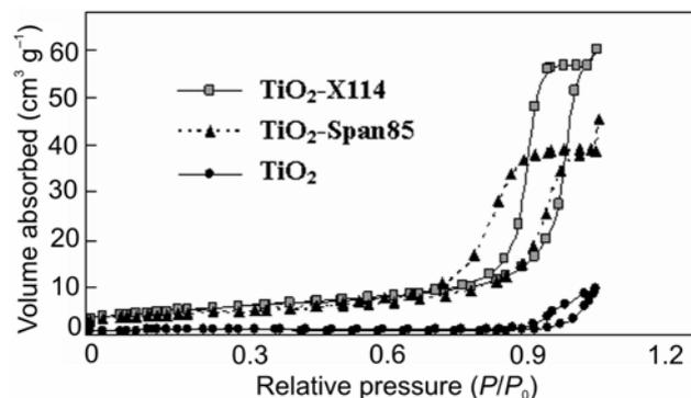
Figure 2. N<sub>2</sub> adsorption/desorption isotherms of TiO<sub>2</sub>-X114, TiO<sub>2</sub>-Span85 and TiO<sub>2</sub>.
