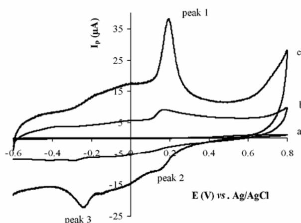
**Figure 2.** Cyclic voltammograms of  $2.00 \times 10^{-5}$  M levodopa at (a) bare GCE, (b) poly(2,5-diaminobenzenesulfonic acid)/GCE and (c) poly(2,5-diaminobenzenesulfonic acid)- $\beta$ -cyclodextrine/GCE in 0.1 M PBS at pH 7.2. Equilibrium time: 5 s, scan rate: 50 mV/s.
