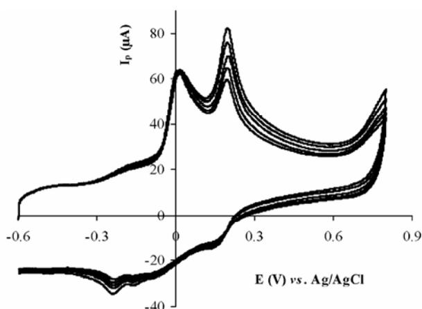
**Figure 7.** Cyclic voltammograms of the mixture of  $3.00 \times 10^{-4}$  M ascorbic acid and increasing concentrations of levodopa at poly(2,5-diaminobenzenesulfonic acid)- $\beta$ -cyclodextrine/GCE in 0.1 M PBS at pH 7.2. Levodopa concentrations: (a)  $3.75 \times 10^{-5}$  M, (b)  $4.25 \times 10^{-5}$  M, (c)  $4.75 \times 10^{-5}$  M, (d)  $5.25 \times 10^{-5}$  M and (e)  $6.00 \times 10^{-5}$  M. Equilibrium time: 5 s, scan rate: 50 mV/s.
