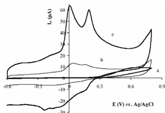
**Figure 6.** Cyclic voltammograms of the mixture of  $3.00 \times 10^{-4}$  M ascorbic acid and  $3.75 \times 10^{-5}$  M levodopa at (a) bare GCE, (b) poly(2,5-diaminobenzenesulfonic acid)/GCE and (c) poly(2,5-diaminobenzenesulfonic acid)- $\beta$ -cyclodextrine/GCE in 0.1 M PBS at pH 7.2. Equilibrium time: 5 s, scan rate: 50 mV/s.
