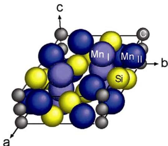
**Figure 1.** Hexagonal uni-cell of the  $Mn_5Si_3$ -type structure with Mn located at two inequivalent Mn sites ( $Mn_I$  and  $Mn_{II}$ ) and carbon arranged along chains through the center of  $Mn_{II}$  octahedra.
