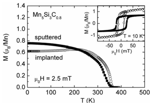
**Figure 2.** Magnetization  $M(T)$  of magnetron sputtered (closed symbols) and  $C^+$ -ion implanted (open circles)  $Mn_5Si_3C_{0.8}$  films. Insets show  $M(H)$  loops taken at  $T = 10$  K.
