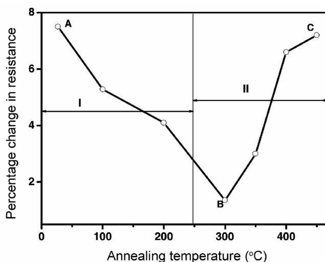
**Figure 2.** Hydrogen sensing response of Cu/Pd bimetal layer at 100%  $H_2$  concentration and at different annealing temperatures.
