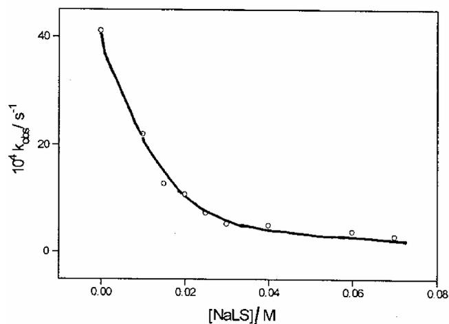
**Figure 2.** Effect of [NaLS] on the rate of base catalysed hydrolytic cleavage of ethyl  $\alpha$ -cyanocinnamate (temperature = 30°C; [NaOH] = 0.001 M).
