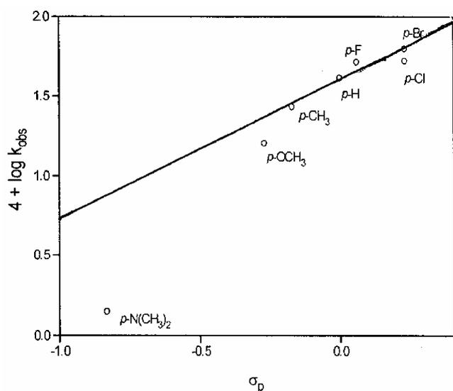
**Figure 1.** Hammett plot for the base catalysed cleavage of *para*-substituted ECC in the absence of surfactant (temperature = 30°C; [NaOH] = 0.001 M).
