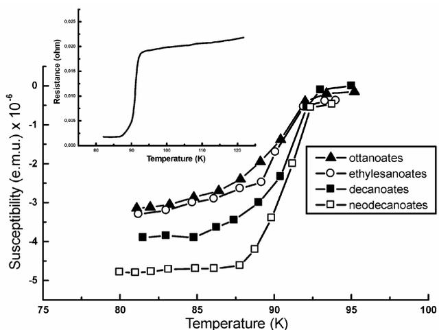
**Figure 8.** Change of magnetic susceptibility as a function of the temperature for YBCO films obtained on MgO substrate starting from different precursors. In the inset the curve of resistance vs the temperature for YBCO sample obtained from neodecanoates is shown.
