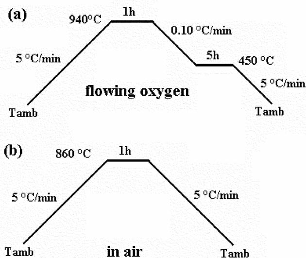
**Figure 2.** Second heat step procedure for YBCO (a) and BSCCO films (b).
