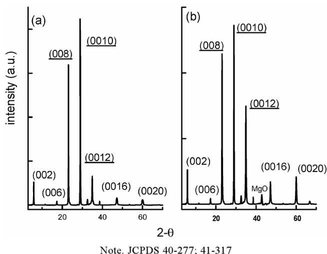
**Figure 5.** XRD spectra of BSCCO samples obtained on Ag (a) and MgO (b) substrates starting from neodecanoates.
