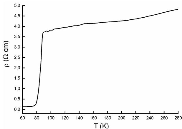
**Figure 7.** Curve of resistance vs. the temperature for Bi-2212 sample obtained on MgO from neodecanoates.
