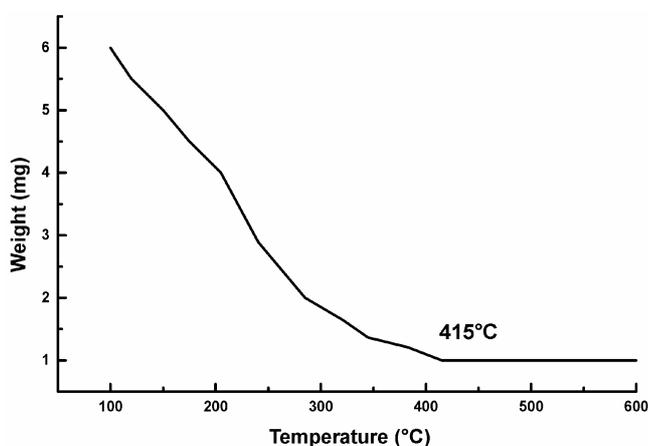
**Figure 1.** TGA result of the film obtained spraying the neodecanoates solution used to synthesize Y-123 samples.
