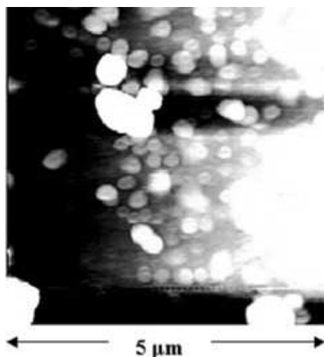
Figure 5. A contact mode AFM picture showing the iron nanoparticles as a 2-dimensional projection. The length of one edge is marked.
