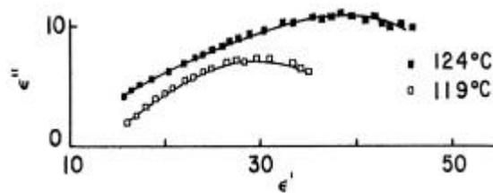
**Figure 4.** Cole–Cole plots for densified (by 1.13%) and undensified glass of composition 21.4  $\text{Na}_2\text{O}$ , 7.2  $\text{Al}_2\text{O}_3$ , 71.4  $\text{SiO}_2$  (mole%) obtained at a temperature of  $120^\circ\text{C}$ .<sup>19</sup>  $\square$  Densified;  $\blacksquare$  undensified.
