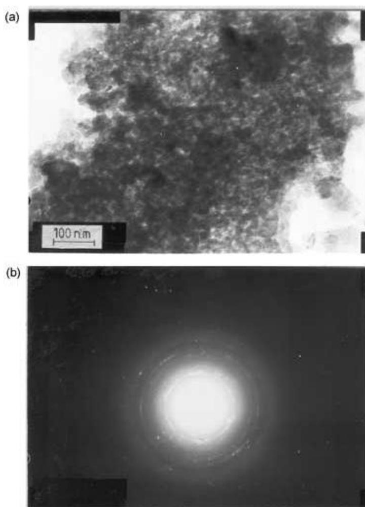
**Figure 1.** (a) Transmission electron micrograph for specimen prepared by reducing the precursor gel at  $650^\circ\text{C}$  for 30 min followed by oxidation at  $700^\circ\text{C}$  for 30 min. (b) Electron diffraction pattern for figure 1a.
