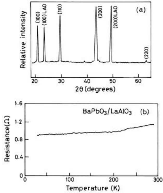
**Figure 5.** (a)  $q$ - $2q$  XRD pattern of BaPbO<sub>3</sub> shows (1 0 0) and (1 1 0) orientations on LaAlO<sub>3</sub> (1 0 0) substrate. (b) Resistance vs temperature plot of BaPbO<sub>3</sub>.
