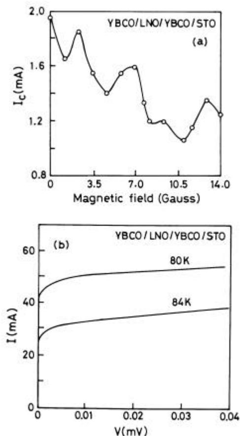
**Figure 4.** Illustration of DC Josephson effect of YBCO/LNO/YBCO/STO Josephson junction. (a) Oscillations of critical current in the applied magnetic field can be seen from the plot. (b)  $I$ - $V$  characteristics at different temperatures.
