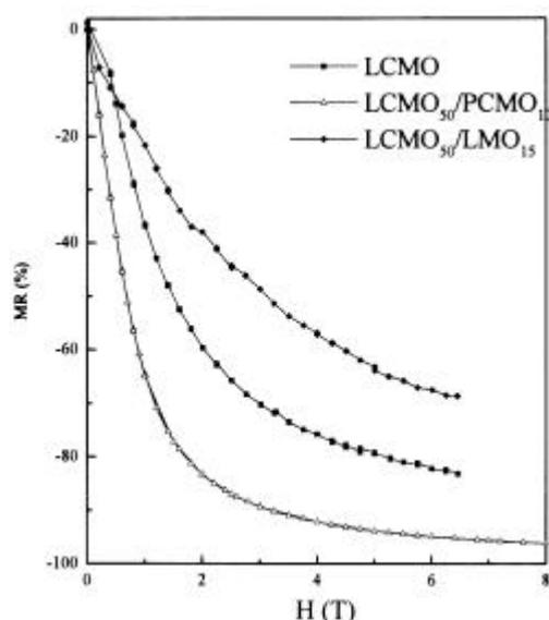
**Figure 8.** The plots of magnetoresistance as a function of applied magnetic field for the LCMO single layer film and LCMO/LNO, LCMO/PCMO multilayers. The curves represent the maximum observed magnetoresistance near their transition temperature.
