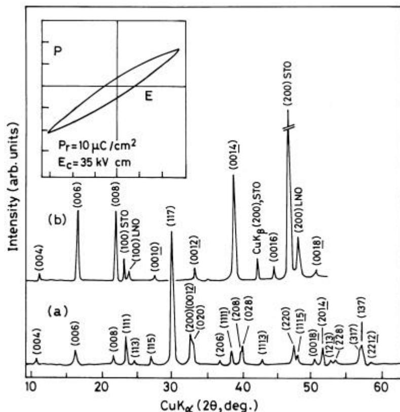
**Figure 7.** XRD patterns of (a) bulk polycrystalline  $\text{Bi}_4\text{Ti}_3\text{O}_{12}$  and (b)  $\text{Bi}_4\text{Ti}_3\text{O}_{12}$  thin film grown on epitaxial  $\text{LaNiO}_3/\text{LaAlO}_3$  (100) film. Inset shows the room temperature ferroelectric hysteresis loop of  $\text{Au}/\text{Bi}_4\text{Ti}_3\text{O}_{12}/\text{LaNiO}_3/\text{LaAlO}_3$  (100).
