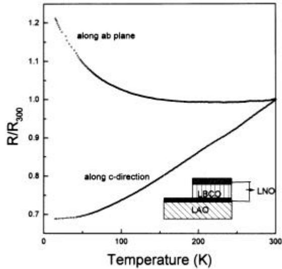
**Figure 6.** Normalized resistance vs temperature plot of LBCO measured along  $a$ - $b$  plane and  $c$ -directions are shown. Inset shows the schematic representation of the thin film structure employed for the  $c$ -direction resistance measurement.
