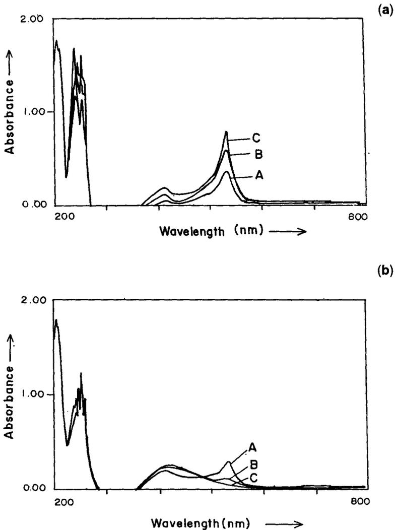
**Figure 1.** Visible spectrum in the presence of stoichiometric amounts of (a) BAPP:Ce(IV) [1:0.25(A), 1:0.50(B), 1:1.00(C)] and (b) BAPP:Ce(IV) [1:1.50(A), 1:2.00(B), 1:3.00(C)].
