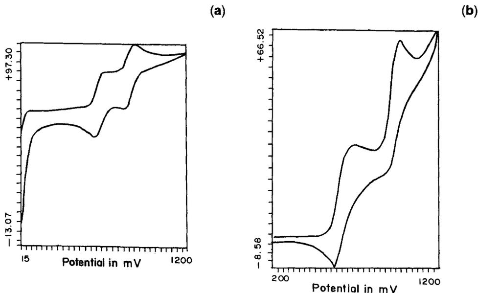
**Figure 3.** Cyclic voltammogram of (a) parent phenoxazine and (b) 10-[3'-N-benzylaminopropyl]phenoxazine.
