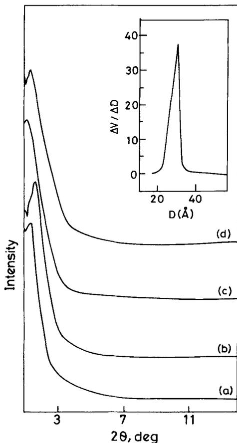
**Figure 1.** X-ray diffraction patterns of alumina prepared with (a) dodecylamine and (b) hexadecylamine as templates. The diffraction patterns of the corresponding calcined samples are shown in (c) and (d) respectively. The inset shows the pore size distribution in a calcined sample (prepared with dodecylamine).
