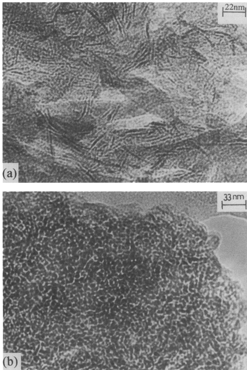
**Figure 2.** Transmission electron microscopic images (a) of the as-prepared alumina (with dodecylamine) and (b) of the calcined sample.
