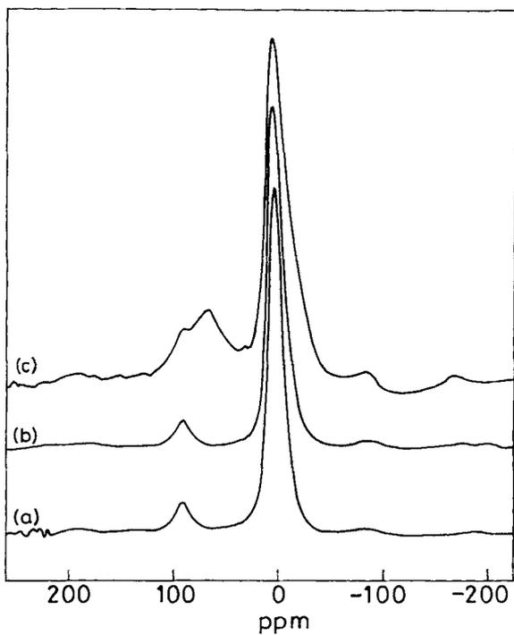
**Figure 3.**  $^{27}\text{Al}$  MASNMR spectra of the alumina samples (a) prepared with dodecylamine, (b) of the dehydrated sample and (c) of the calcined sample.
