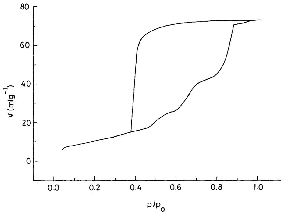
**Figure 4.**  $\text{N}_2$  adsorption-desorption isotherm of the calcined alumina (with dodecylamine).
