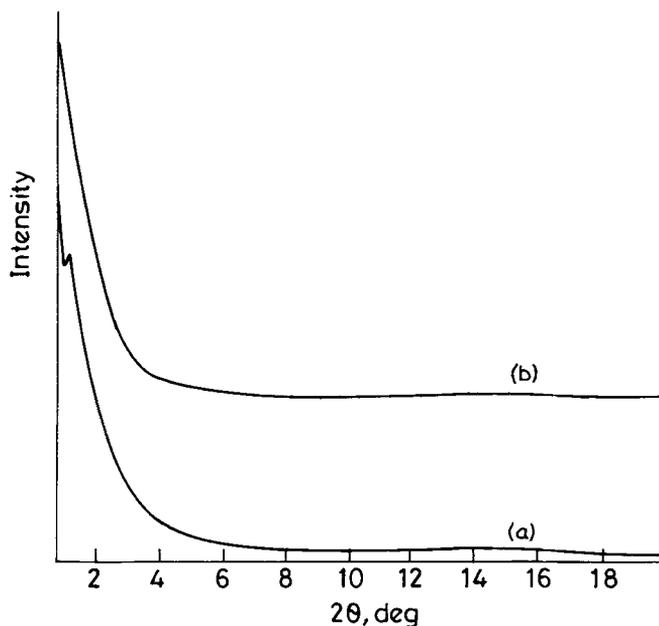
**Figure 5.** X-ray diffraction patterns of alumina prepared with (a) Tween 80 (b) hexylamine.
