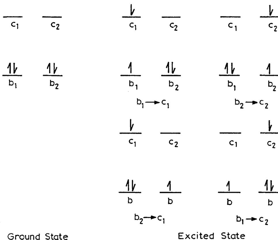
**Figure 3.** Schematic diagram of frontier orbital description of porphyrins.
